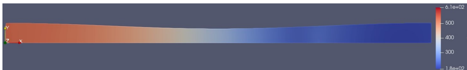
Figure B.21: Contour of the static pressure field for the case with wall friction and heat convection.
