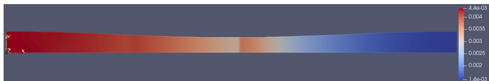
Figure 6.75: Contour of the density field (SI values) for the channel with L = 150m .
