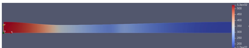
Figure B.13: Contour of the static pressure field for the channel case with a throat located at x_{throat}/L = 0.25 .
