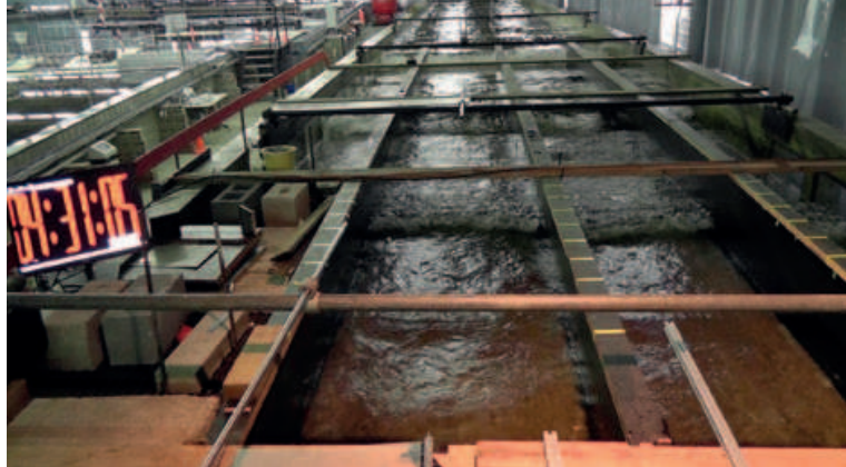
Figure 3. Image of flume in Antwerp: wave breaking on the foreshore (photo courtesy Xuexue Chen).
