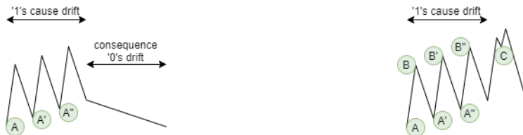
(a) Consecutive '1's cause an upward trend. As a consequence, when '0's are transmitted right after a sequence of consecutive '1's, they tend to drift as well, in order to get back to symbol A.
