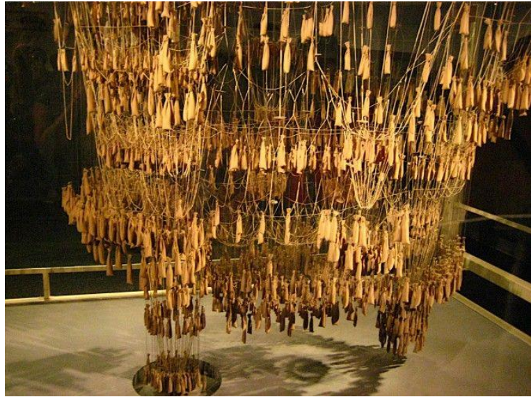
Figure 03.3 Hanging chain model of Sagrada Familia by Antoni Gaudi [Source: pinterest.com ]
