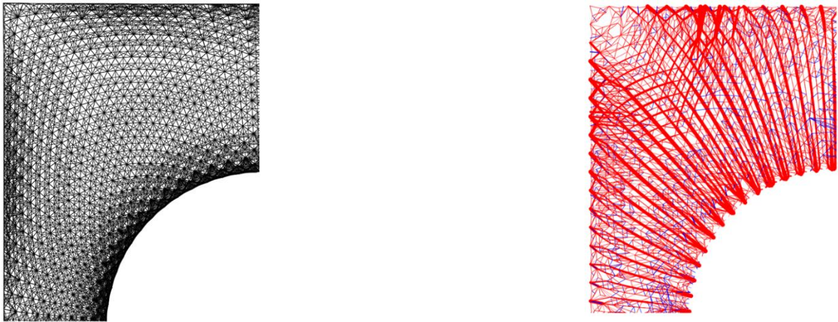
Figure 04.7 Ground structure (left) and Optimized layout (right) [4]
