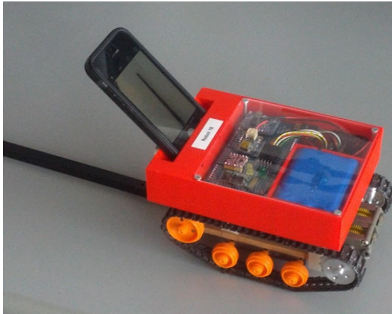
Figure 5.4: Diagram of line-follower robot
