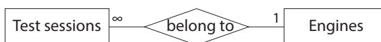
Figure 6.2: A one-to-many relation between the engine entity and the test session entity.
