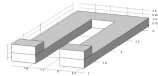
(b) Single-turn coil | Cross-section of 0.1x0.3m
