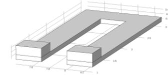
(c) Single-turn coil | Cross-section of 0.05x0.3m
