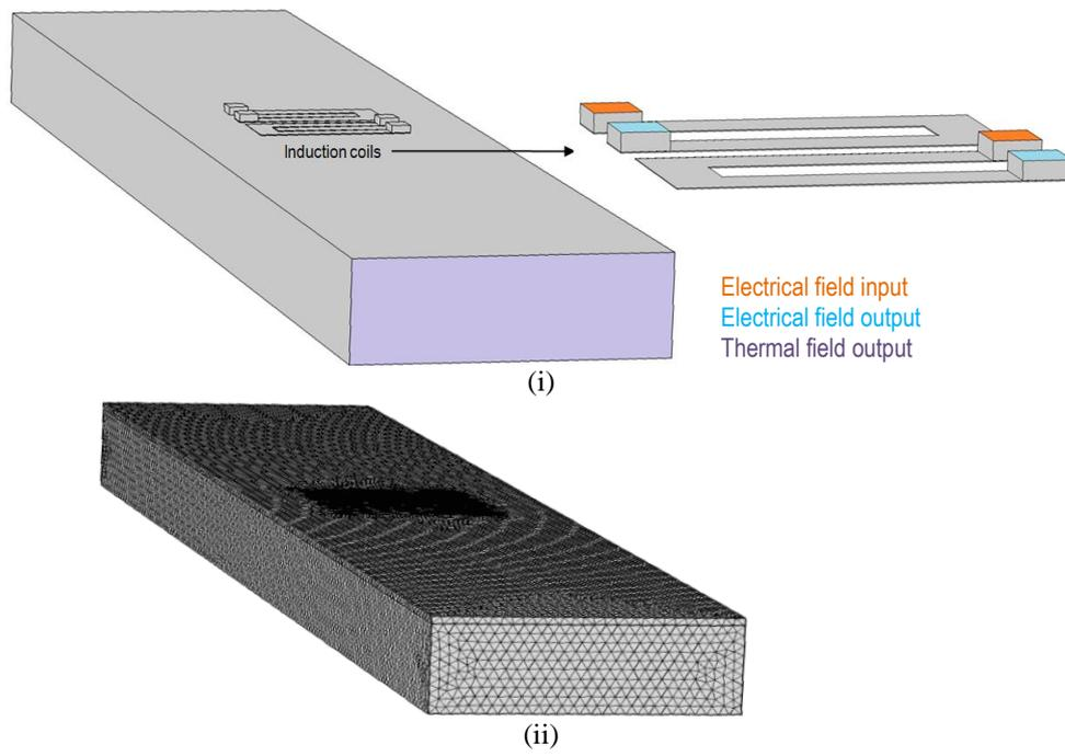
**FIGURE 2 (i) Three-dimensional geometry and (ii) mesh of induction heating system**
