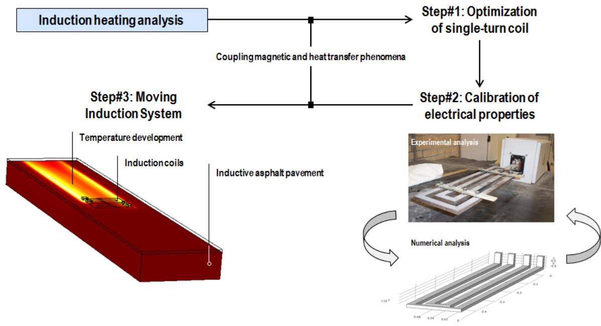
**FIGURE 3 Methodology for induction heating analysis**
