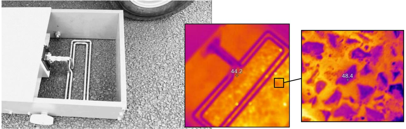
**FIGURE 1 Induction heating of motorway A58 in the Netherlands (June 2014)**
