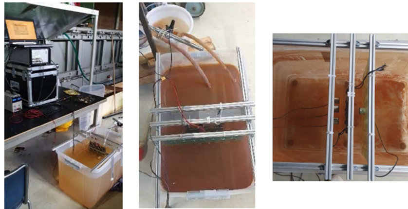
Figure 5. Accelerated corrosion experiments setup.
