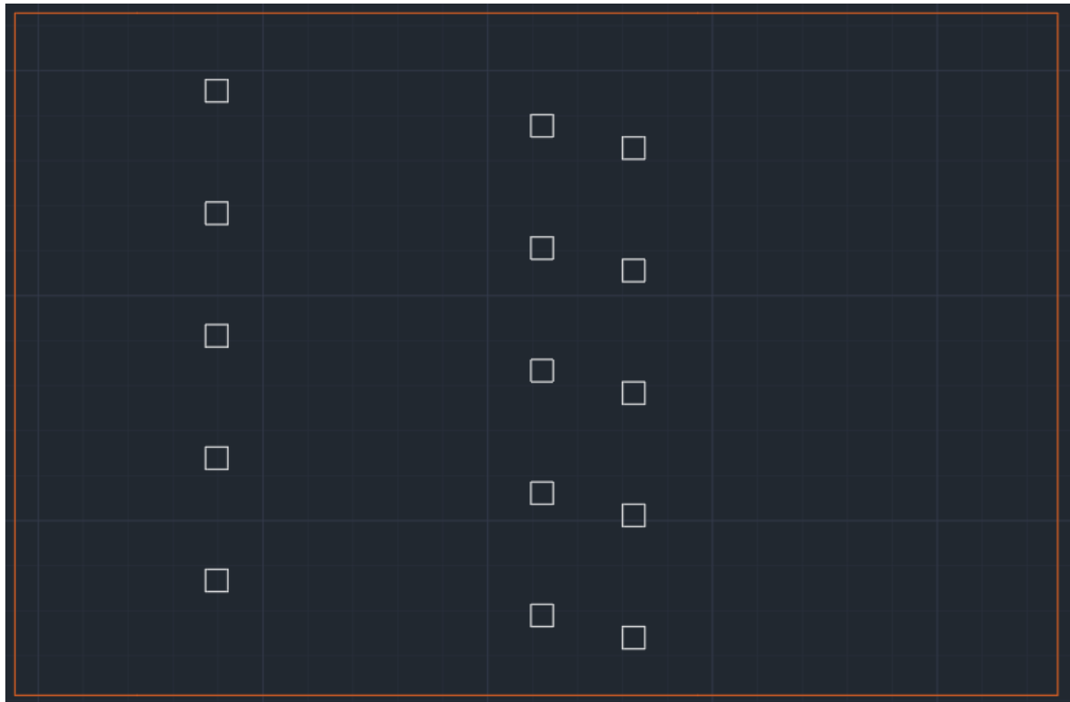
Figure D.8: Mask Wafer_2_Front_Side_Tube_hole used in step 12 of Wafer2 in Appendix C. The image shows a single chip. The mask defines the holes in the front side silicon nitride membrane where the microtubes will connect. The orange lines are not part of the actual mask and only show the borders of the chip. The width of the orange box is 14500 \mu\text{m} .
