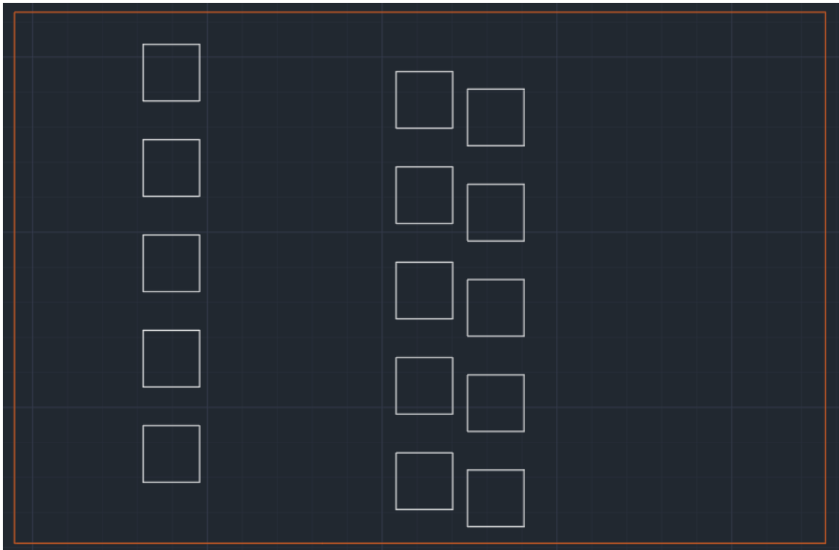
Figure D.2: Mask Wafer_1_Back_Side_Tube_hole used in step 13 of Wafer1 in Appendix C. The image shows a single chip. The squares show the through-wafer holes of the deep reactive ion etching. The orange lines are not part of the actual mask and only show the borders of the chip. The width of the orange box is 14500 \mu\text{m} .
