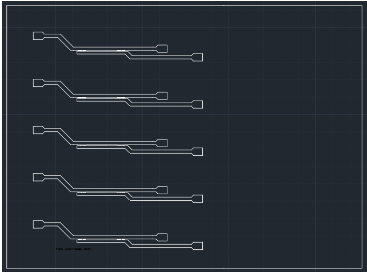
Figure D.10: Mask Wafer_3_Front_Side_Microfluidics used in step 5 of Wafer3 in Appendix C. The image shows a single chip. The microfluidic inlet ports (left side) and outlet ports (right side) are clearly visible.
