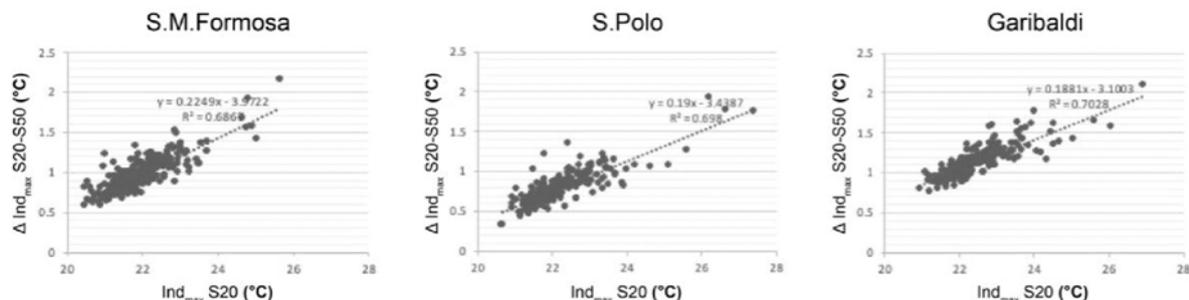
**Figure 4:** Correlation between maximum indoor temperature in S20 and increase of maximum indoor temperature in S50
