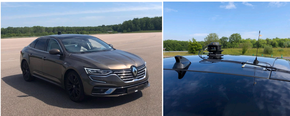
Fig. 1. The experimental vehicle, a Talisman phase 2 (left), with the VBOX GPS antenna (right).
