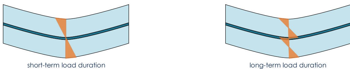
Figure 0-6: Section through laminated glass indicating bending stress within plies for short-term and long-term conditions.
