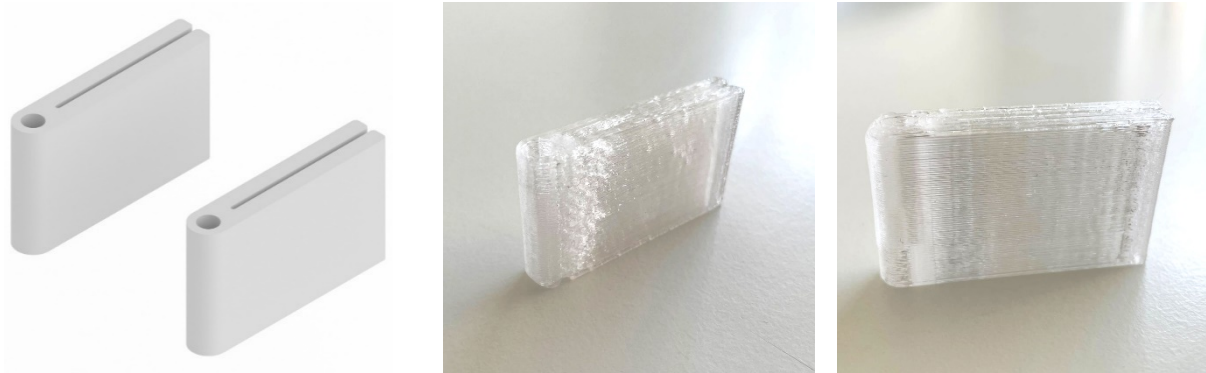
Figure 2-43: Capture of the .stl file, ready to be 3d-printed (left) and the actual 3d-printed connections, made from PETG (mid and right). (own).
