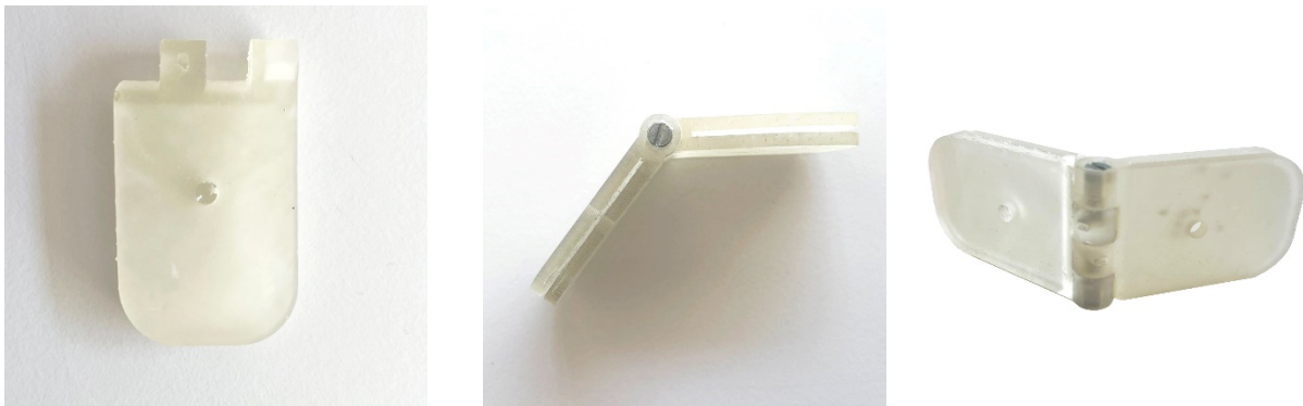
Figure 2-44: 3d printed connections using uv treated clear resin. The detail in such a method is higher (own).
