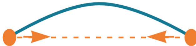
Figure 2-17: Tension is needed from the sides so the panel could be held bent in place (own illustration).
