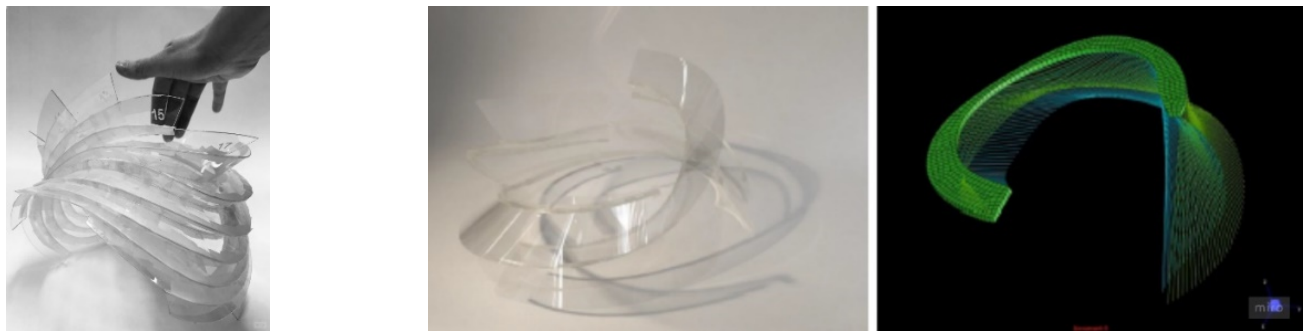
Figure 1-17: Photographs of the ultra-thin glass structure in different design stages and a simulation using Strand7 (Pennetier & Stoddard, 2019).
