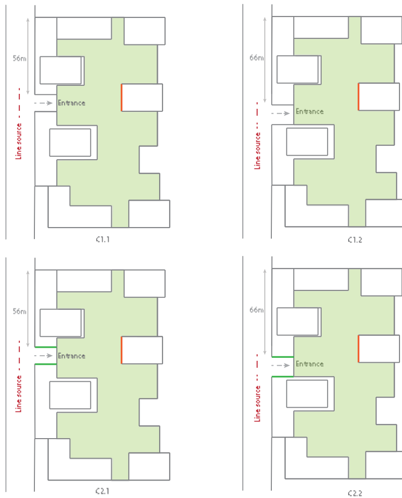
Figure 87 Courtyard sequences. C1.1: Entrance at 56m (Base case), C1.2: Entrance at 66m (10m offset case), C2.1: Base case with green wall at entrance, C2.2: 10m offset case with green wall at entrance
