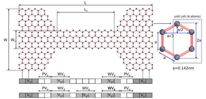
Fig. 1. Butterfly Graphene Nanoribbon (GNR).
