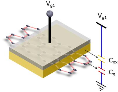
Fig. 5. Top gate capacitance.
