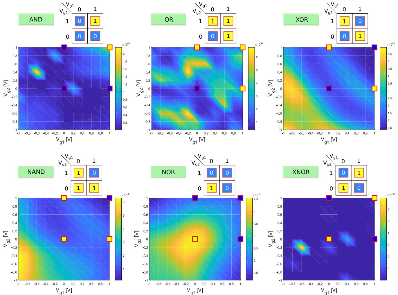
Fig. 3. 2-input boolean functions conduction maps.
