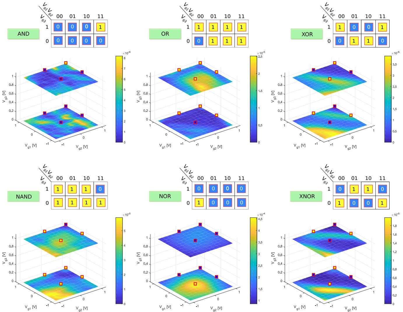
Fig. 4. 3-input boolean functions conduction maps.
