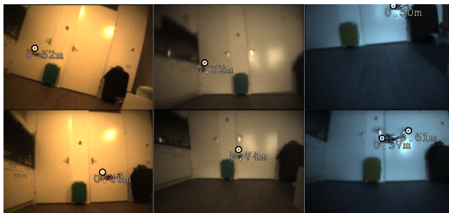
Fig. 8: Testing results of the refined network on randomly selected testing images. The white circle in images shows the predicted pixel position of peer robot center. The value on the image means the depth of the robot from the camera. All testing images are captured onboard with different flying attitude and velocity of both quadrotor, captured at different day times.
