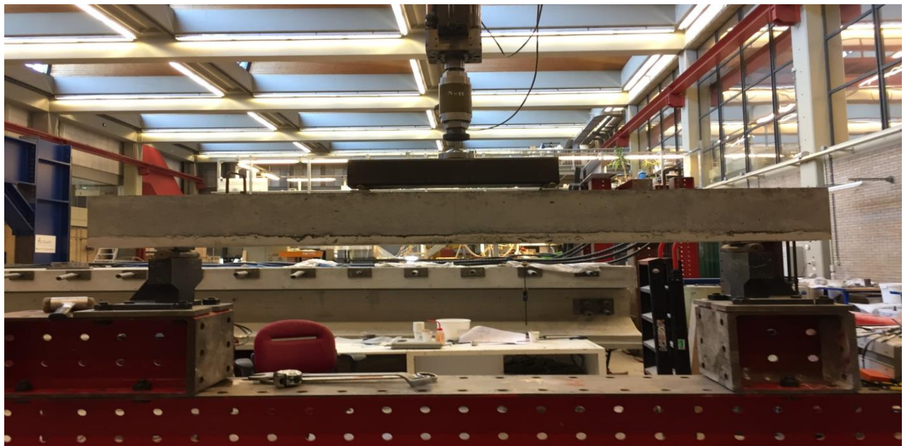
Figure 2.2 Experimental Setup of the Four Point Bending Test Performed by Mr. Zhekang Huang.
