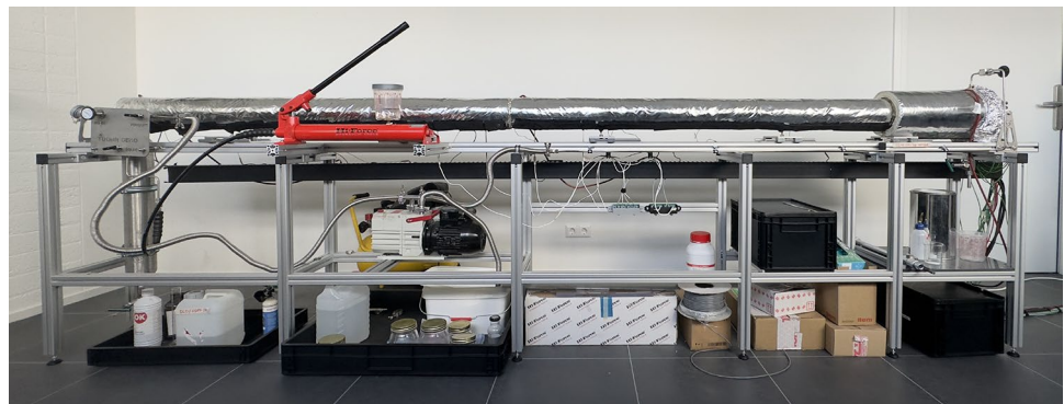
Fig. 3 Photograph of the ASTER setup. The charge tube and the low pressure tank are covered with glass-silk heating jackets
