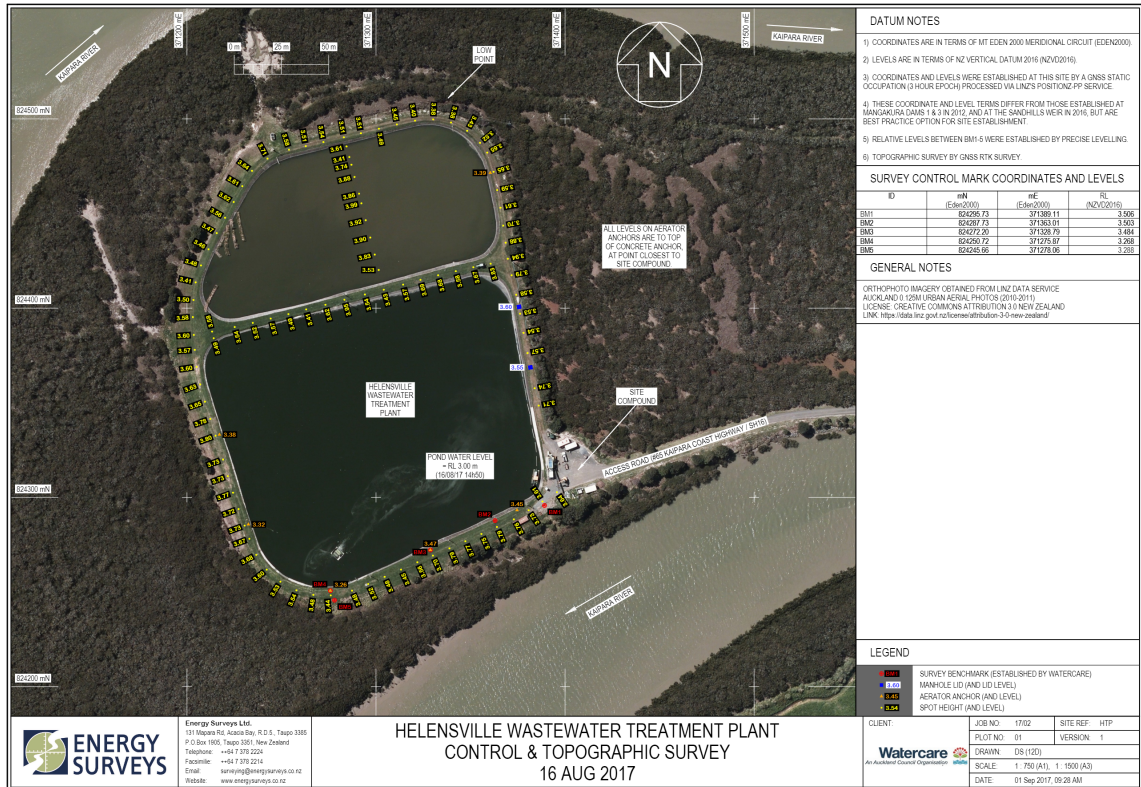
Figure C.6: Crest elevation of the pond embankments surrounding the wastewater treatment plant (Stephens et al., 2021)
