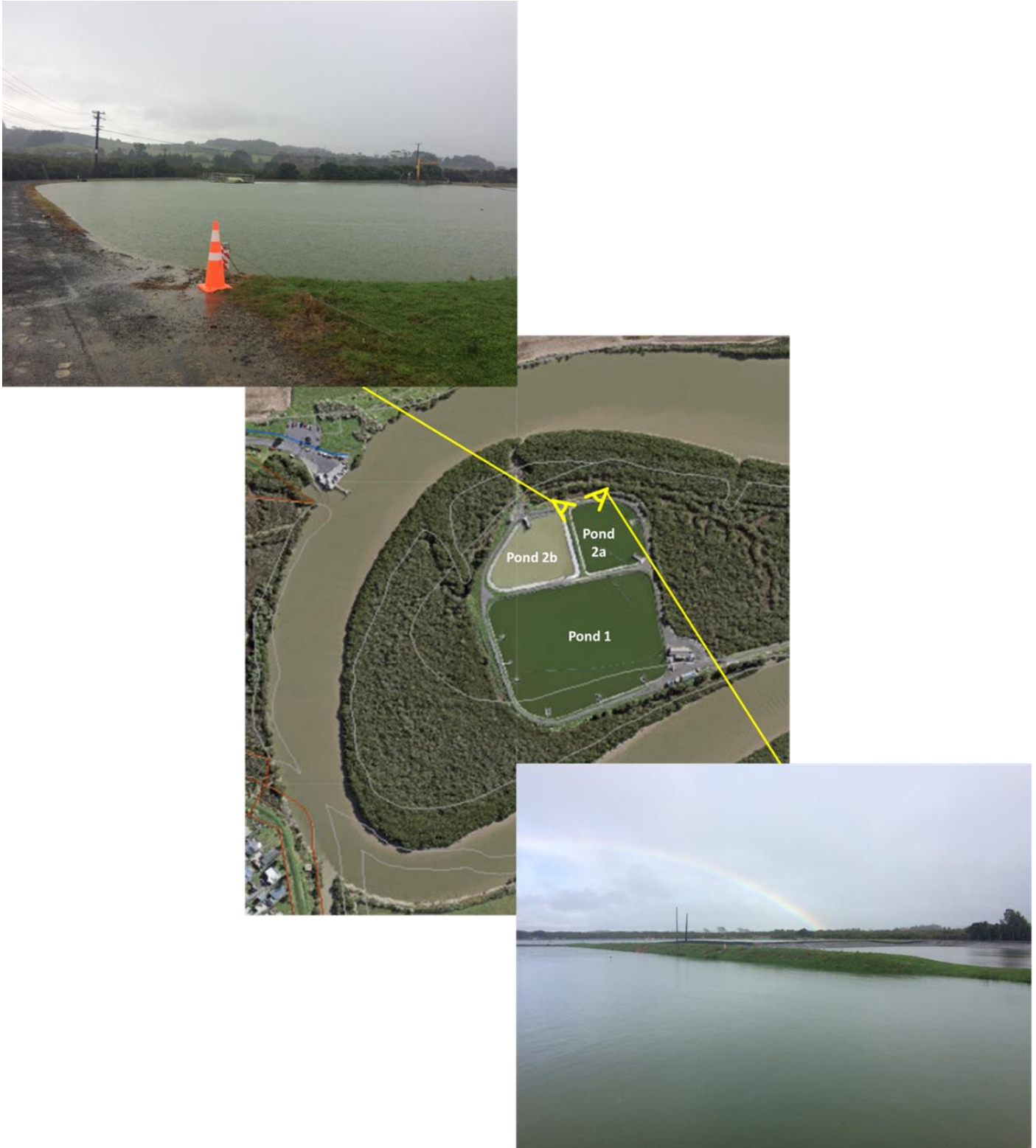
Figure 1: 7 th July 2017 wet weather event (60mm over 2 days). Pond levels at 1815mm. The pond will overtop the dam embankment into the harbour at 1.85m.
