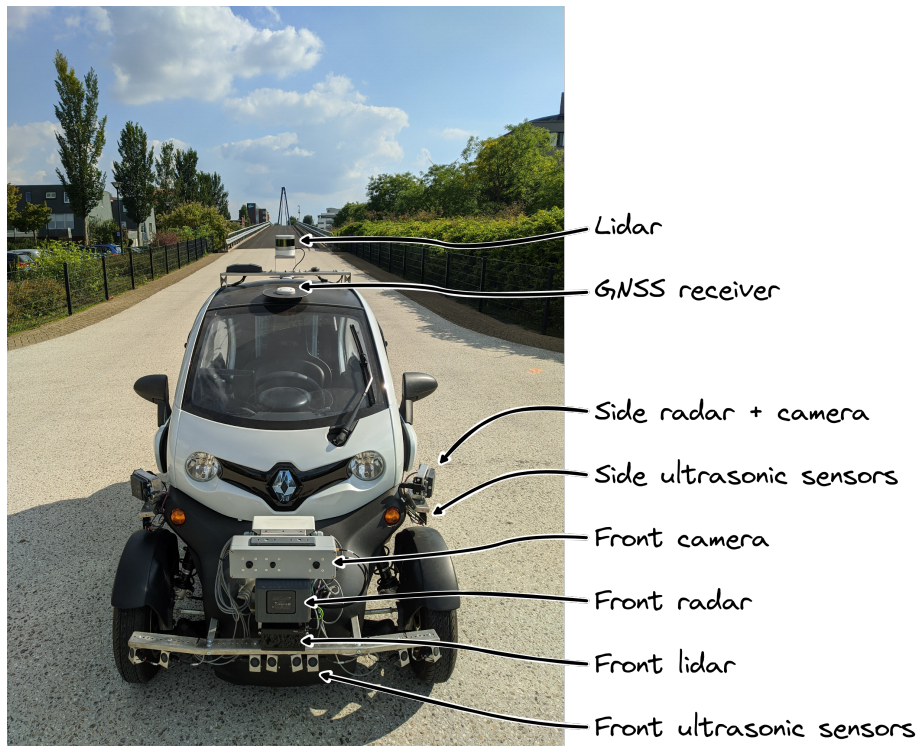
Figure 5.11: Front view of the Twizy R&D vehicle. The Twizy R&D vehicle is a manually driven vehicle equipped with state-of-the-art automotive sensors, which allows it to record datasets of its environment. The sensor set of the Twizy R&D vehicle consist of a roof-mounted lidar, GNSS receiver, front and side facing camera, front and side facing radar, front facing lidar and front and side facing ultrasonic sensors.
