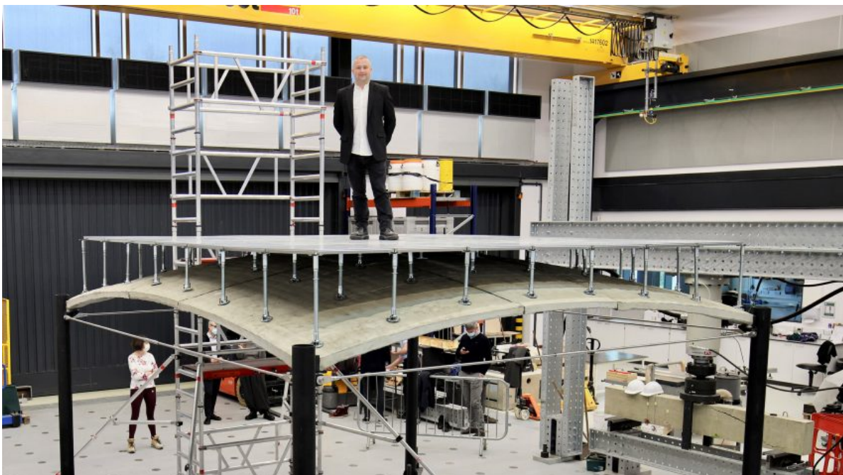
Figure 2.6: Vaulted slab by ACORN [44]
