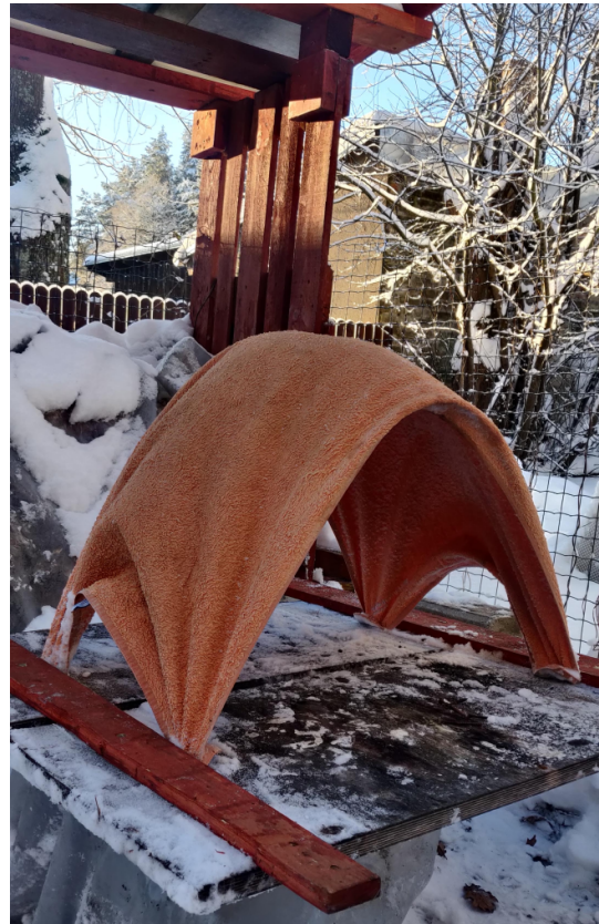
(b) Frozen towel inverted and fixed in a rig
