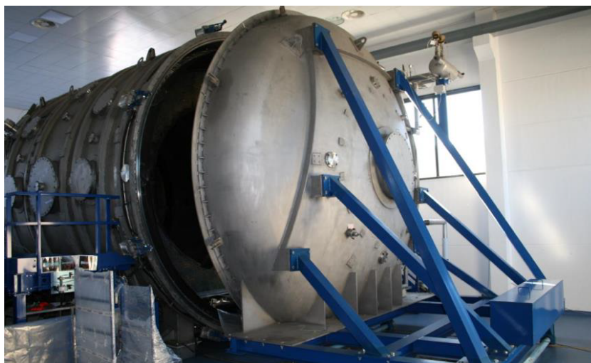
Figure 5.3: SITAEL IV10 vacuum chamber. (Source: Ref [111])
