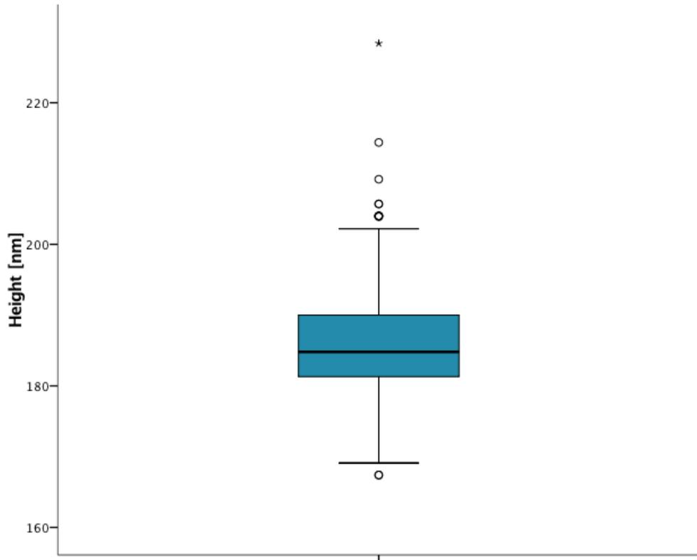
Figure 10: Boxplot of pillar height, showing median, maximum- and minimum values (whiskers) and outliers (°) of all patterns
