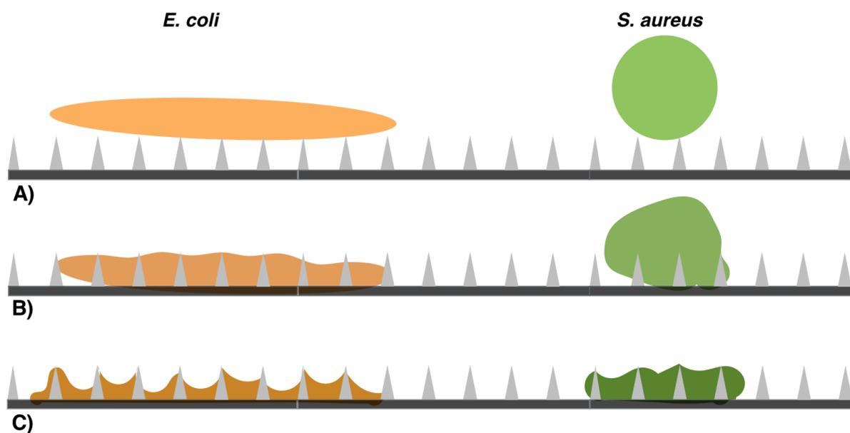
**Figure 7: Schematics of interaction of *E. coli* and *S. aureus* with nanopillars. A) Healthy bacterial cells on pattern B) Deformed bacterial cells on pattern C) Severely deformed bacterial cells on pattern**
