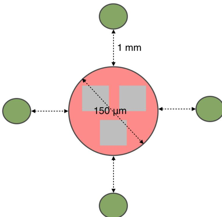
**Figure 6: Inspected areas (on one sample) for analysing morphology, bacterial density and bactericidal efficacy: red area is (close to) patterned surface, green areas are far from patterned area (1 mm distance)**
