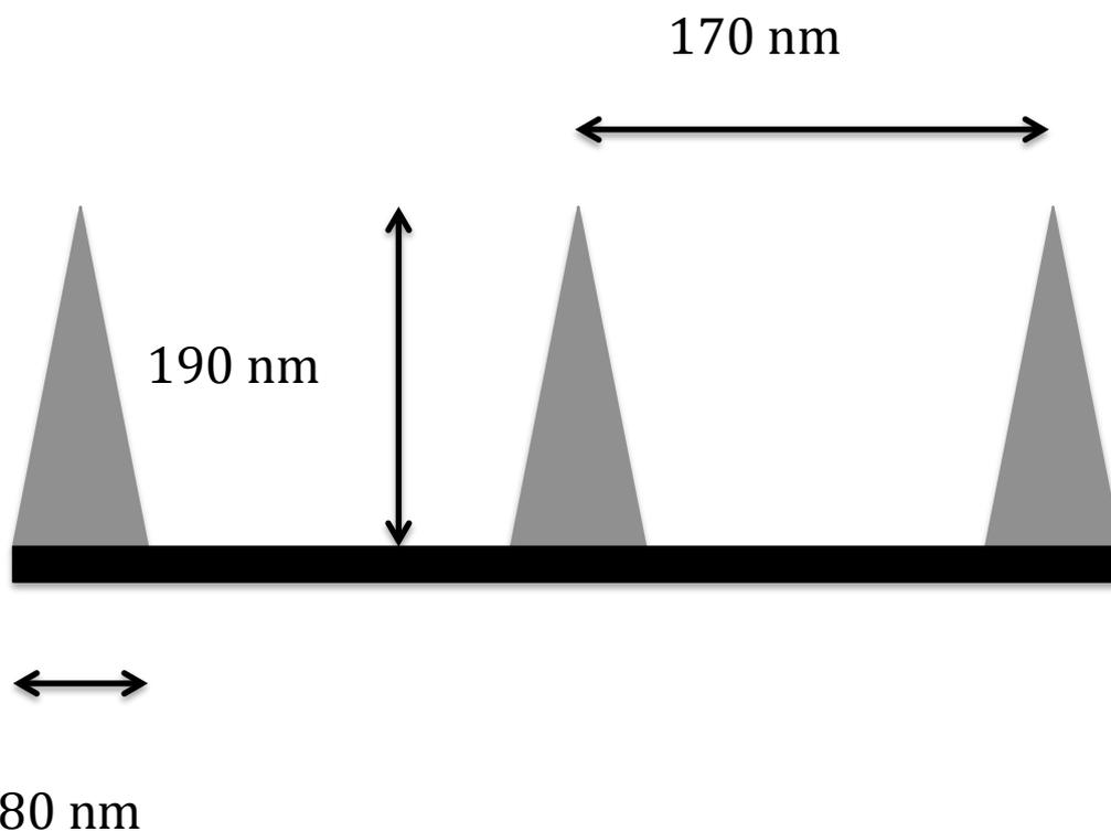
Figure 1: Schematic representation of pillars including diameter, height and interpillar distance
