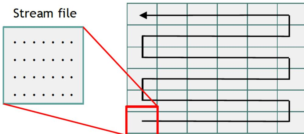
**Figure 4: Serpentine strategy: step and repeat process for increasing the total area of patterning [10].**
