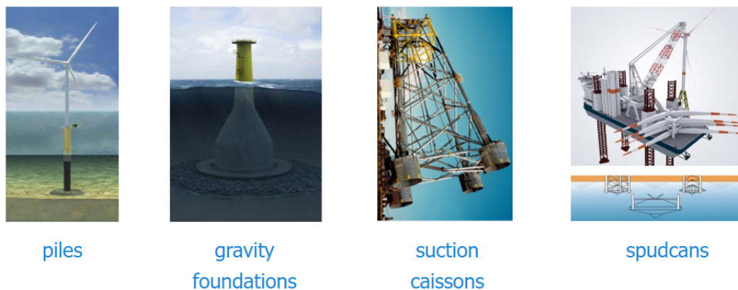
Figure 1.2: Various types of foundations for OWT
