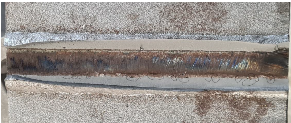
Figure 4.70: Detected crack initiation with simple photography test by TNO [12]
