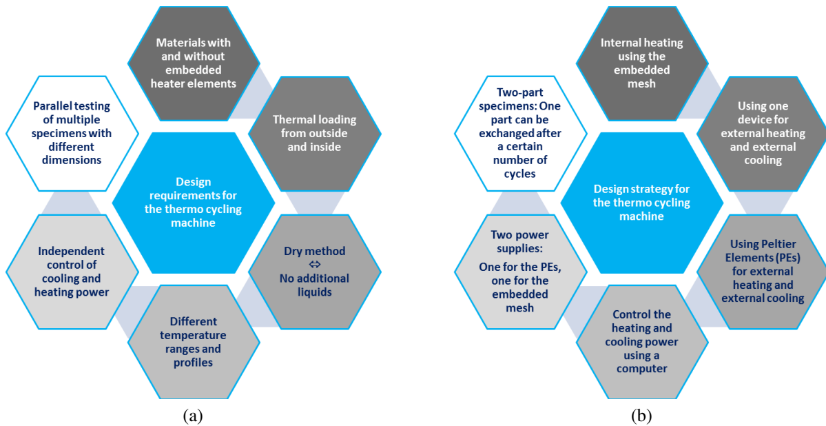
Figure 3. Thermal cycling machine: (a) Design requirements and (b) design strategy (start at the top, proceed clockwise)
