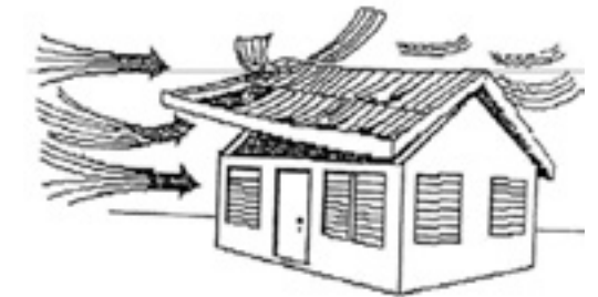
Figure 5 - Improper connection roofing materials (Agarwal, 2007)
