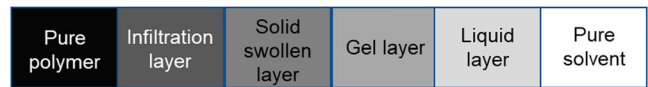
Figure 10. Schematic representation of the surface layer structure, adapted from Miller-Chou and Koenig (2003).
