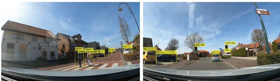
Figure 7. Bounding boxes generated using the YOLOv4 algorithm for Driving Test 5 (left: elapsed time = 1039 s, right: elapsed time = 1400 s). A YOLOv4 model (Bochkovskiy, Wang, and Liao 2020) pretrained on the COCO dataset was used (Lin et al. 2014; obtained from sbairagy-MW 2021).
