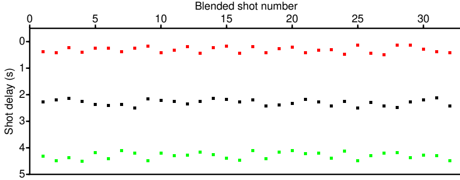
Figure 6.8: The blending code for the streamer example. Each column contains the delay times for a particular blended shot record. Red, black and green dots represent the first, second and third shot respectively.
