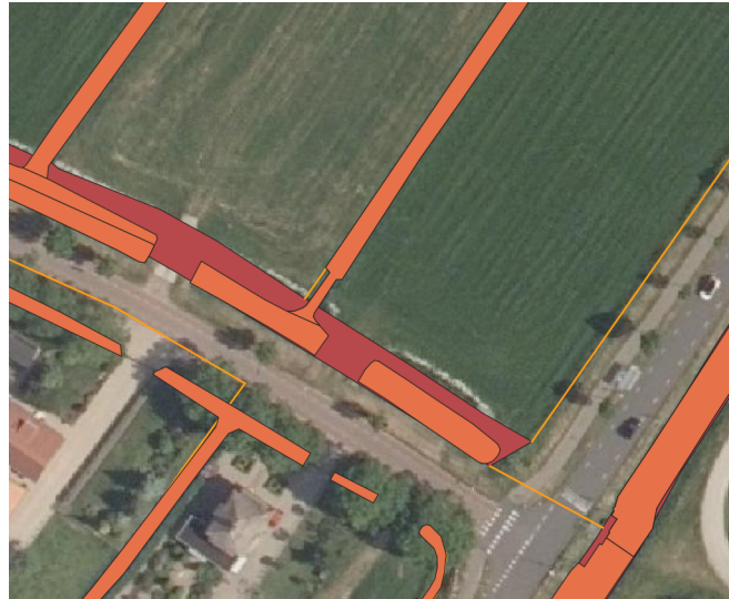
Figure 3.8: Example of differences between BGT Water objects (polygons) and TOP10NL Water objects (lines)
