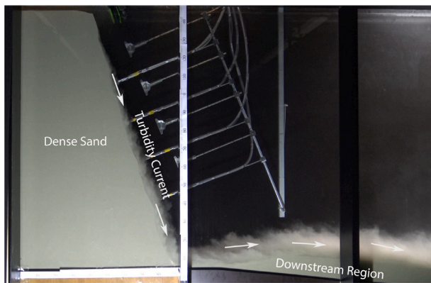
Fig. 5. A breaching experiment in progress; the initial angle of the breach face was 70^\circ (Alhaddad et al., 2020c).
