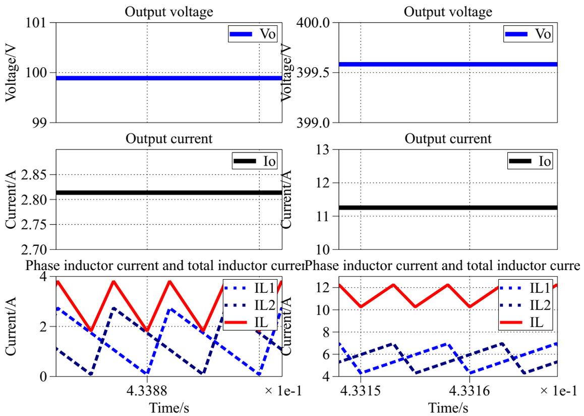
Figure 3.20: Simulation waveforms for designed two-phase interleaved CCM scenario charging on 100 V, 282 W
