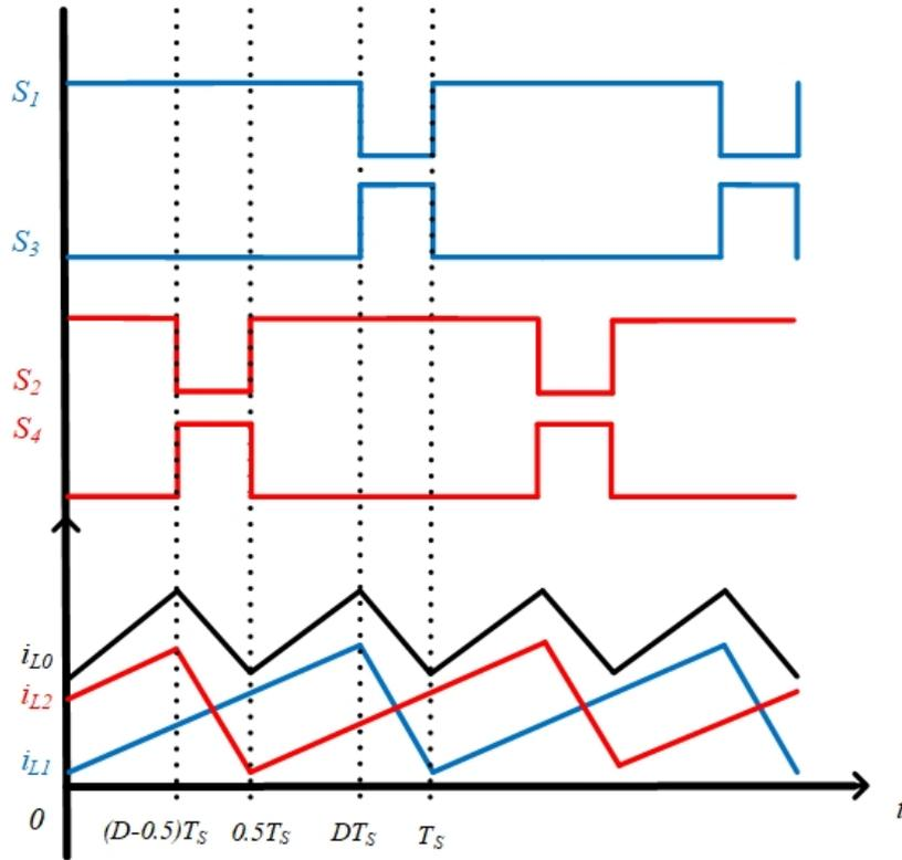
Figure 3.16: Two-phase interleaved buck converter inductor current waveform when  $D \geq 0.5$  in CCM
