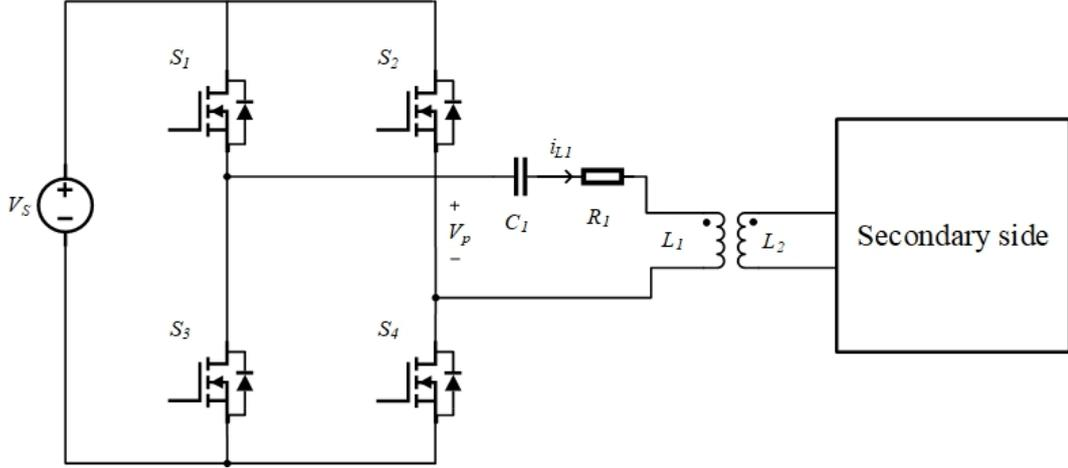
Figure 4.1: Front-end phase shift regulation WPT circuit
