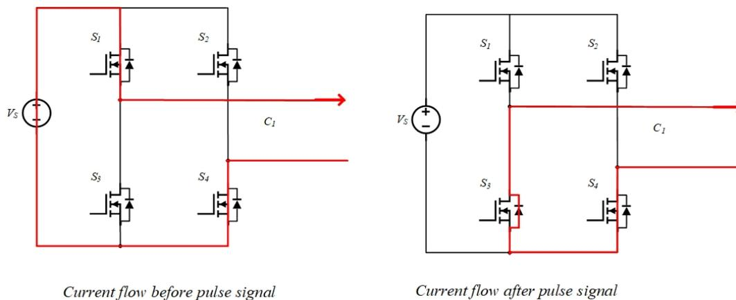
Figure 4.5: Current flow analysis at  $t_2$
