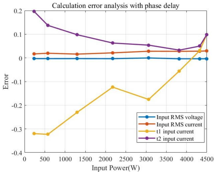
Figure 4.11: Calculation error analysis of phase-shift control with phasedelay
