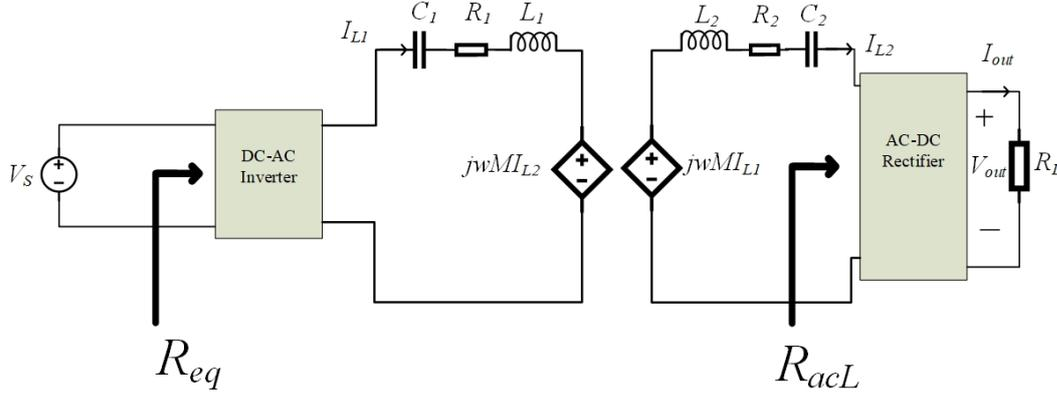
Figure 2.2: WPT circuit with S-S compensation
