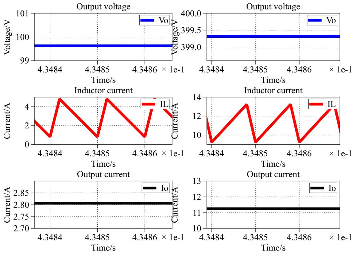
Figure 3.7: Simulation waveforms for designed single phase CCM scenario charging on 100 V, 282 W
