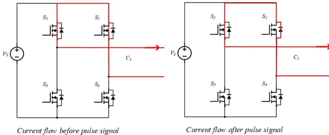
Figure 4.4: Current flow analysis at  $t_1$
