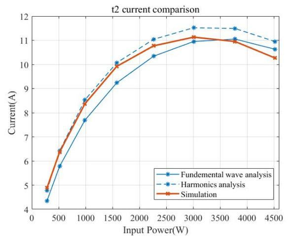
Figure 4.15: Comparison of primary coil current at  $t_2$
