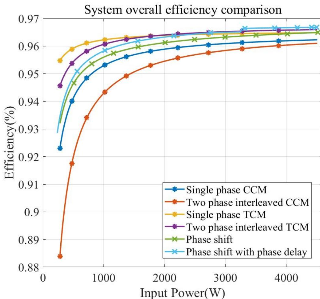
Figure 4.19: System efficiency comparison between all six designed scenarios
