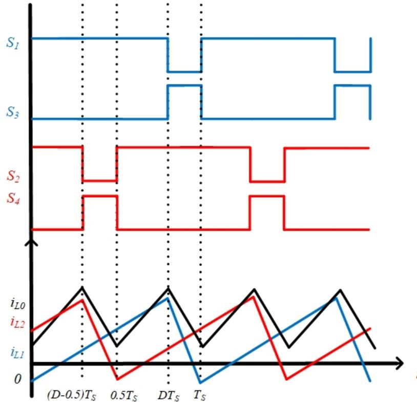
Figure 3.22: Two-phase interleaved buck converter inductor current waveform when  $D \geq 0.5$  in TCM
