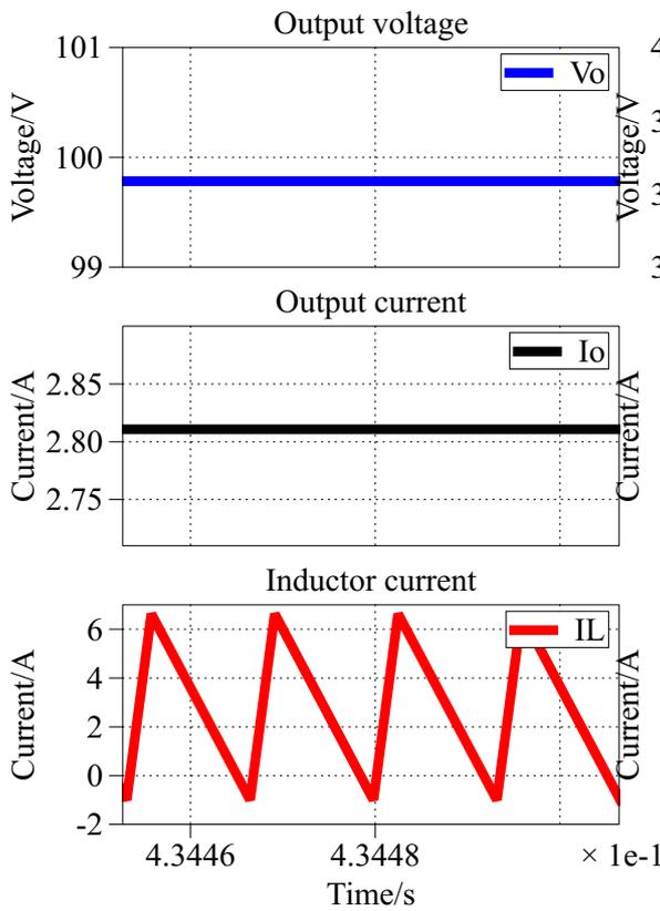
Figure 3.12: Simulation waveforms for designed single phase TCM scenario charging on 100 V, 282 W
