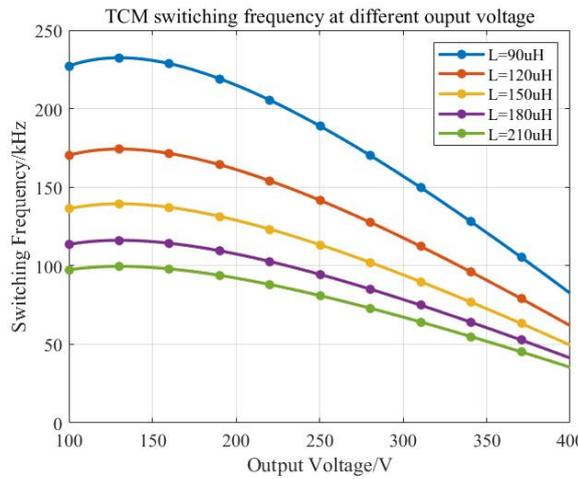
Figure 3.23: Two-phase interleaved buck TCM switching frequency sweeping
