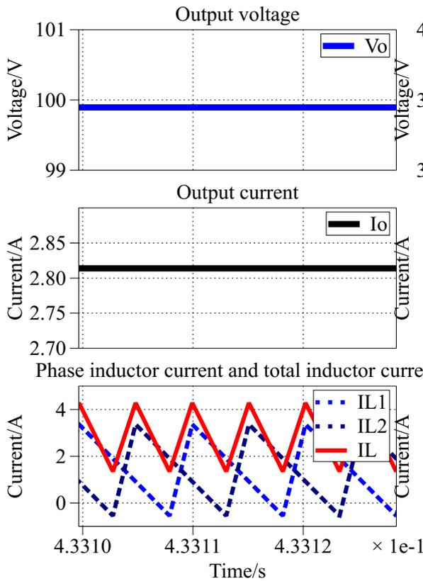
Figure 3.25: Simulation waveforms for designed two-phase interleaved TCM scenario charging on 100 V, 282 W
