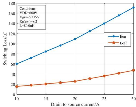
Figure 3.3: Switching loss of SiC MOSFET G3R75MT12J Figure 3.4: Replotted Switching loss datasheet from datasheet
