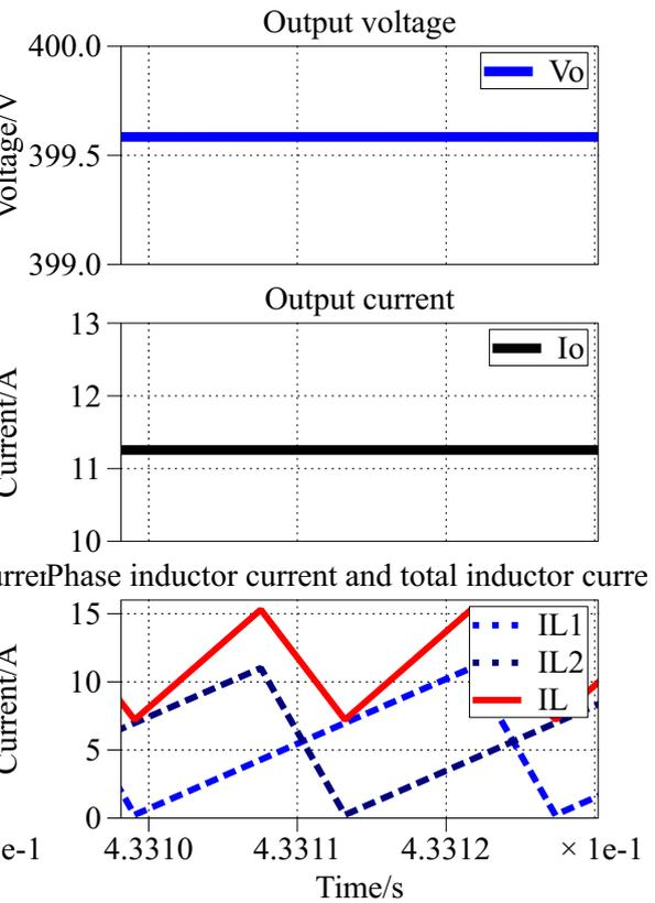
Figure 3.26: Simulation waveforms for designed two-phase interleaved TCM scenario charging on 400 V, 4500 W
