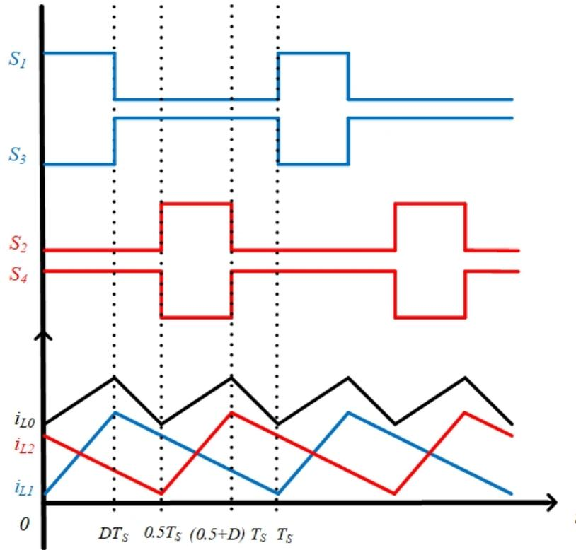
Figure 3.15: Two-phase interleaved buck converter inductor current waveform when  $D < 0.5$  in CCM
