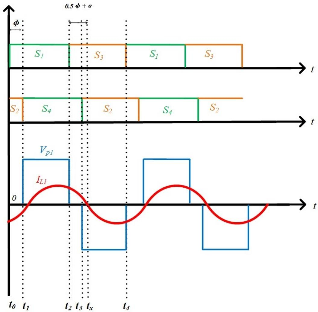
Figure 4.7: Switching sequences and the primary voltage and current waveform of Phase shift control with phase delay
