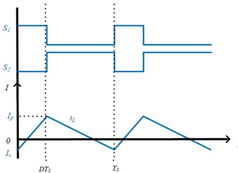
Figure 3.9: Single phase buck inductor current waveform
