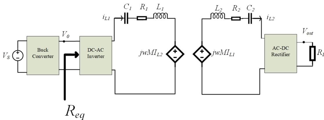
Figure 3.1: Front buck converter WPT structure
