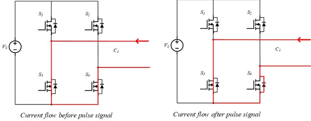
Figure 4.6: Current flow analysis at  $t_3$
