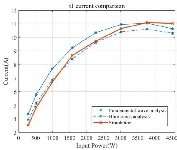
Figure 4.14: Comparison of primary coil current at  $t_1$
