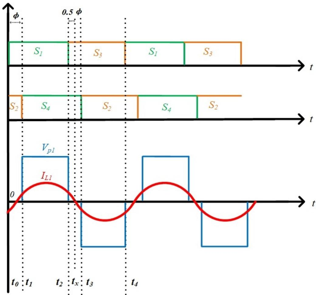
Figure 4.2: Switching sequences and the primary voltage and current waveform of Phase shift control
