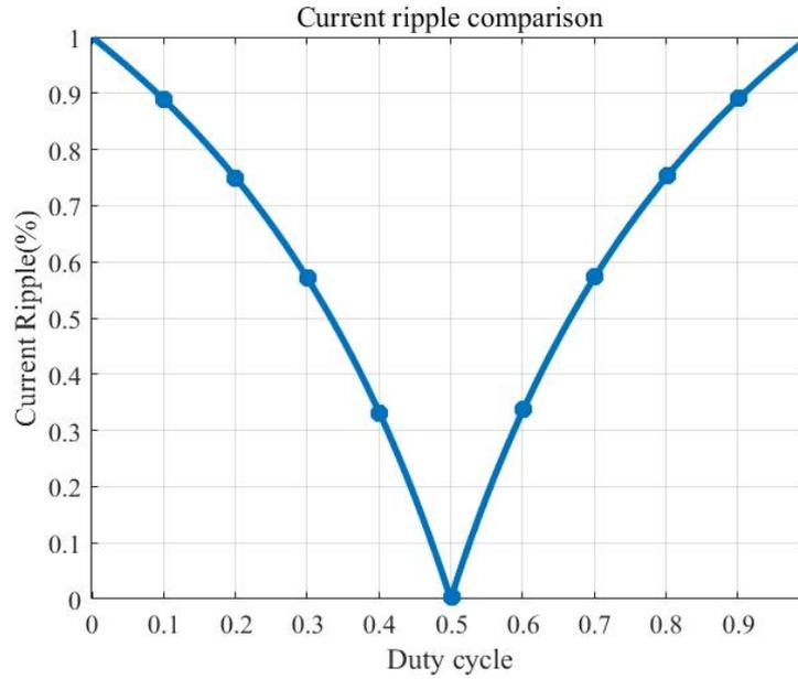
Figure 3.17: The current ripple reduction ratio of the two-phase interleaved output current ripple divided by the single-phase output current ripple
