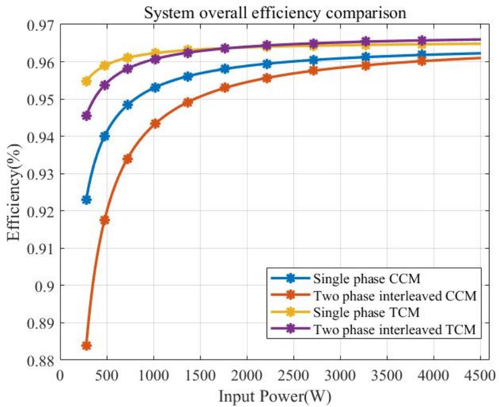
Figure 3.29: System overall efficiency comparison at different power level
