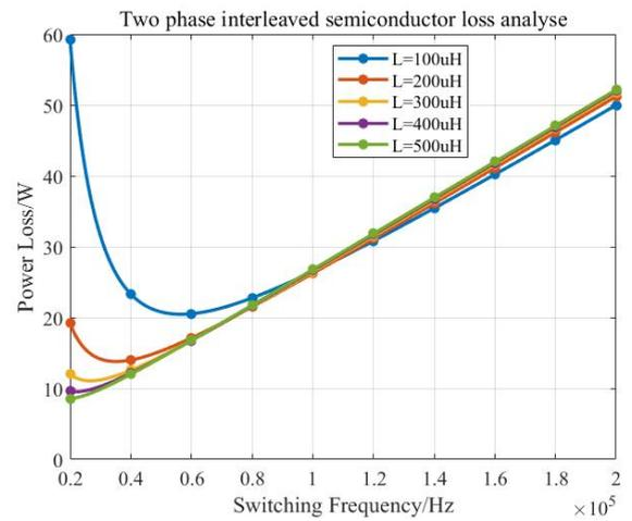
Figure 3.18: Analyses of inductor current ripple with the fre- Figure 3.19: Two-phase interleaved CCM semiconductor losses sweeping hard-switched CCM.
