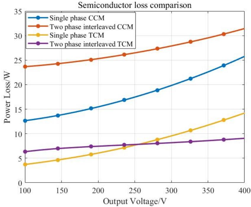
Figure 3.27: Semiconductor losses comparison
