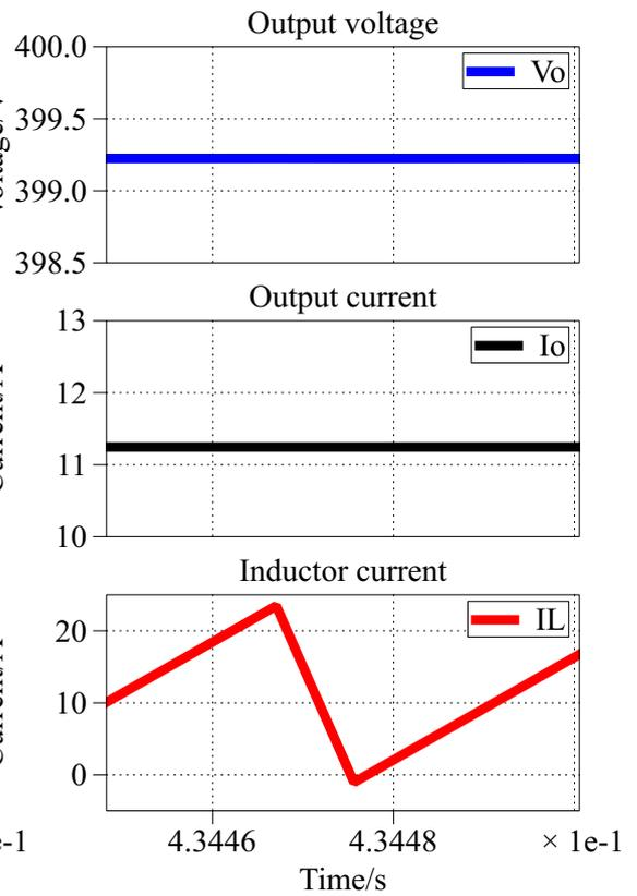
Figure 3.13: Simulation waveforms for designed single phase TCM scenario charging on 400 V, 4500 W
