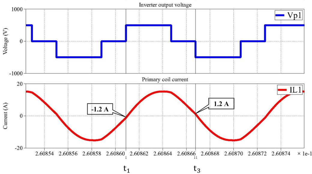
Figure 4.9: Simulation of designed phase shift control without phase delay at the input power of 3152 W
