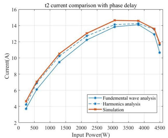
Figure 4.17: Comparison of primary coil current at  $t_2$  with phase delay
