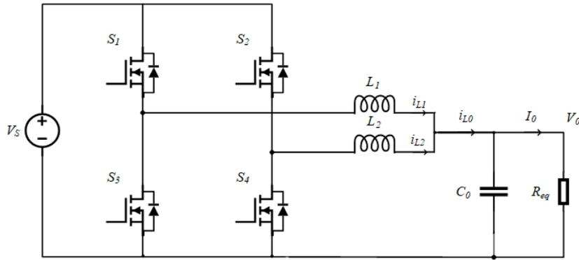
Figure 3.14: Two-phase interleaved buck converter structure
