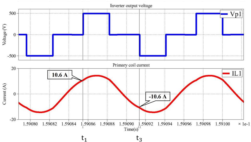
Figure 4.8: Simulation of designed phase shift control at the input power of 3152 W
