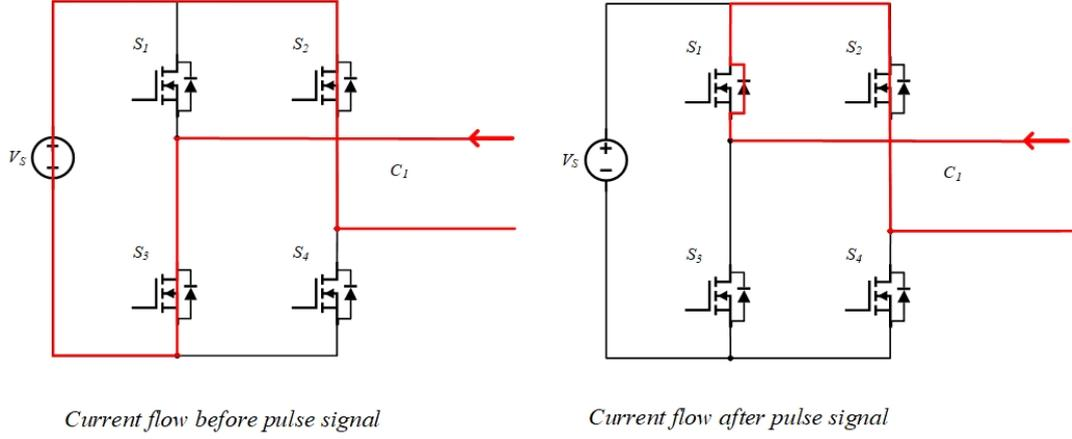
Figure 4.3: Current flow analysis at  $t_0$
