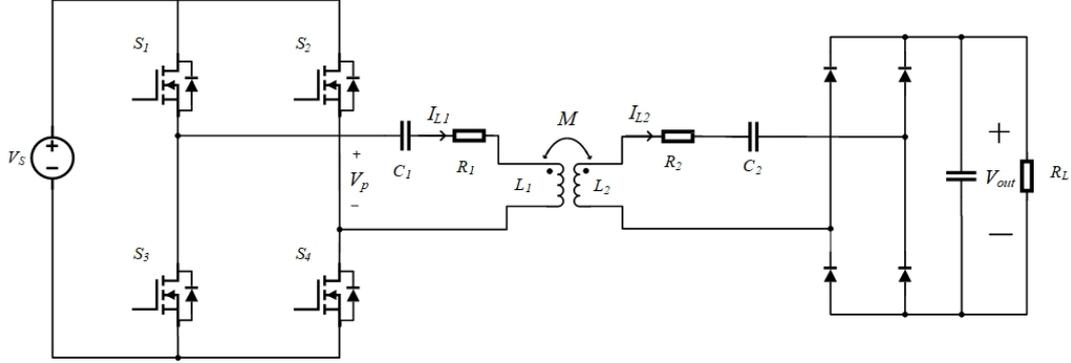
Figure 2.1: WPT circuit with S-S compensation
