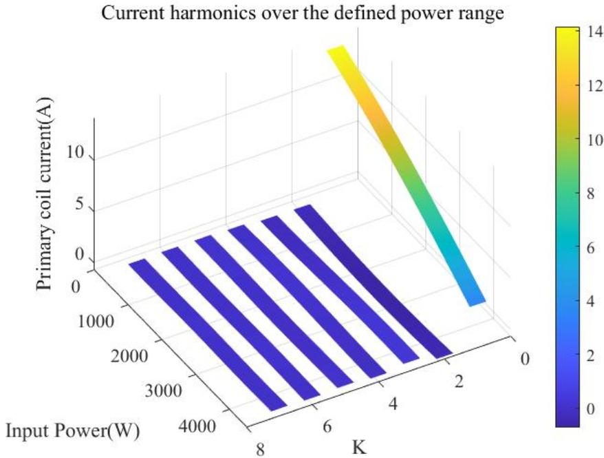
Figure 4.13: Primary coil current harmonics analysis
