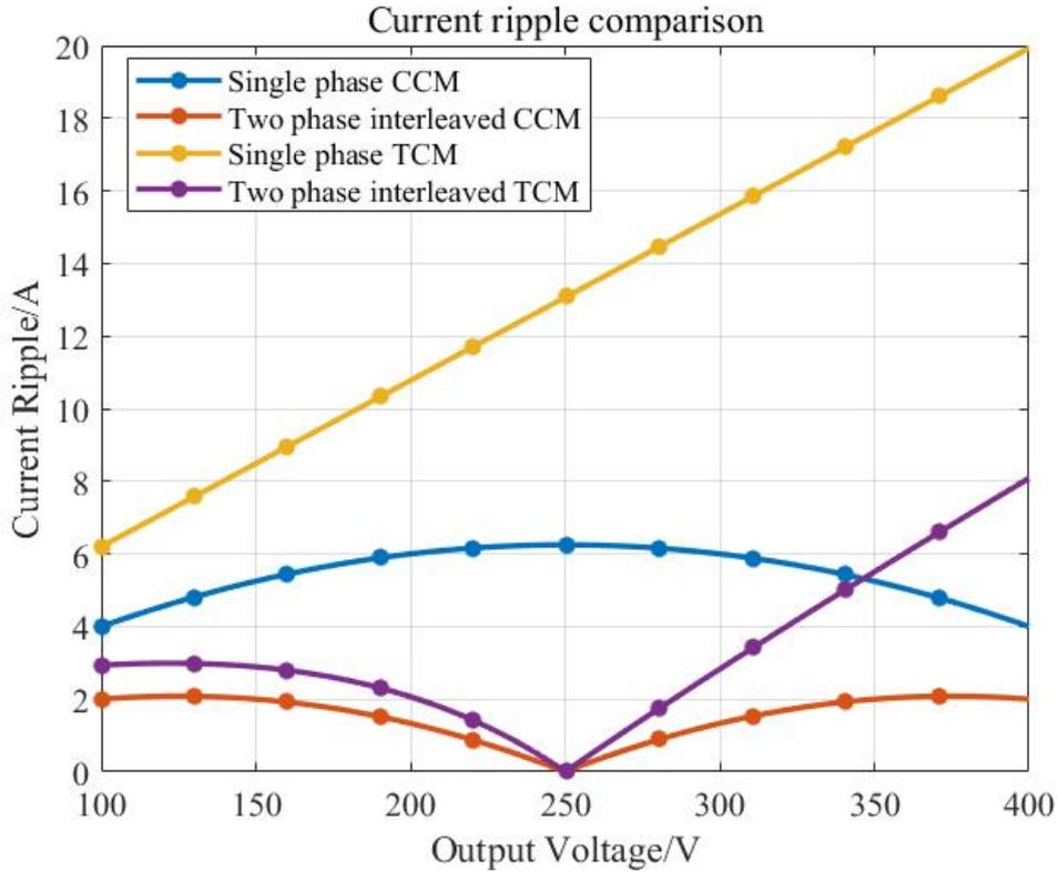
Figure 3.28: Total inductor current ripple comparison
