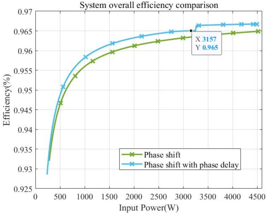
Figure 4.18: Comparison of two scenarios of phase shift methods
