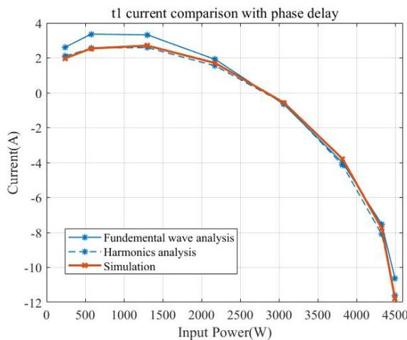
Figure 4.16: Comparison of primary coil current at  $t_1$  with phase delay
