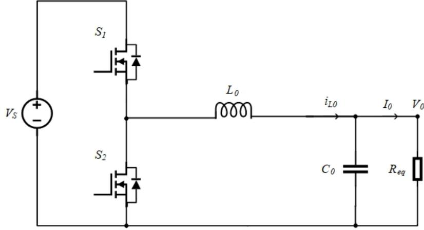
Figure 3.2: Single phase buck converter structure
