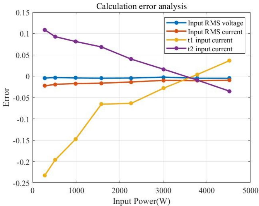
Figure 4.10: Calculation error analysis of phase-shift control without phase delay
