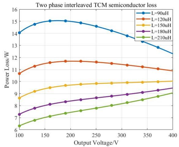
Figure 3.24: Two-phase interleaved buck TCM semiconductor losses sweeping
