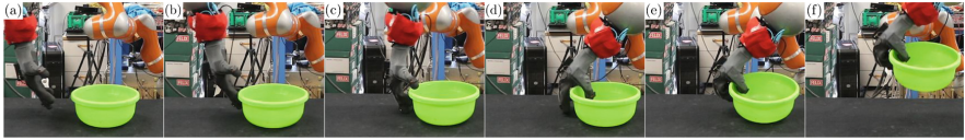
Fig. 5. Photosequence of a grasp produced by the proposed architecture during validation. The hand starts from the initial configuration of the primitive in panel (a). The contact happens in panel (b), triggering the reactive routine. In panel (f) the object is firmly lifted.
