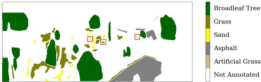
Figure 5-2: Annotation mask; the small details of the sand class within the red boxes are removed in order to assess its influence on the final segmentation.
