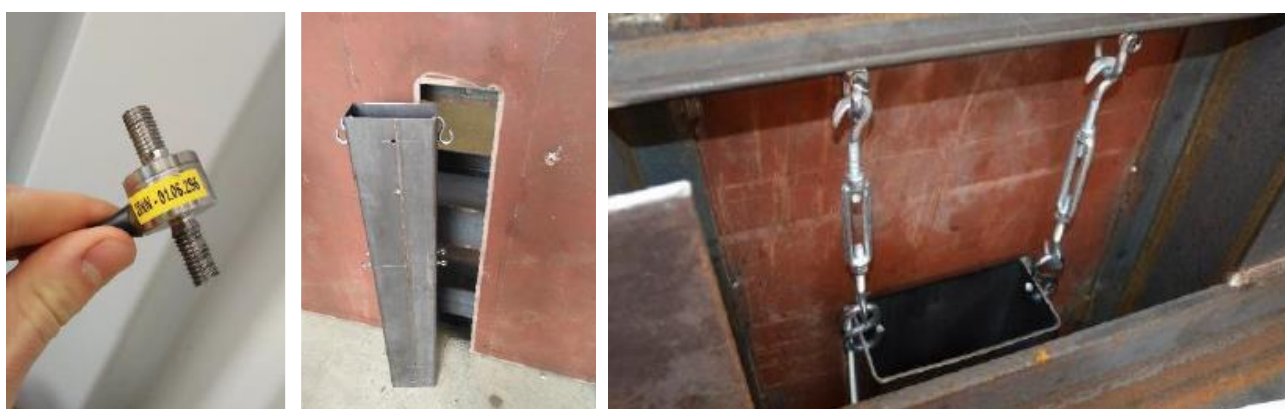
Figure 23: Left: HBM U9 compression load cell. Centre: hollow steel profile and gap in steel wall to accommodate it. Bottom: hollow profile installed, as viewed from behind the steel wall.
