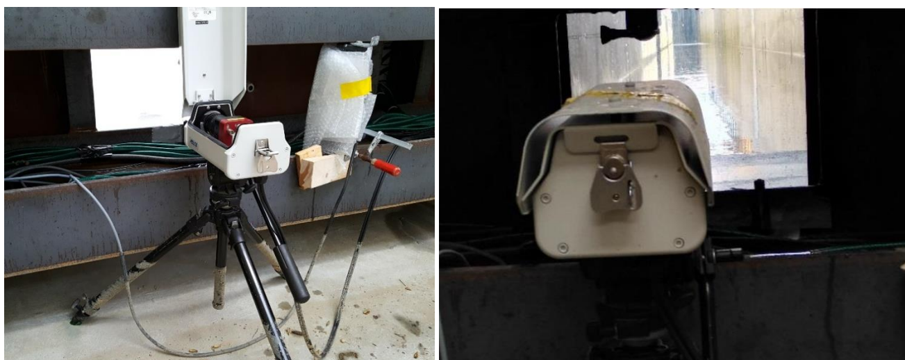
Figure 20: The high-speed camera as mounted behind the promenade wall (left) and approximate view of the camera (right). Camera in protective case.
