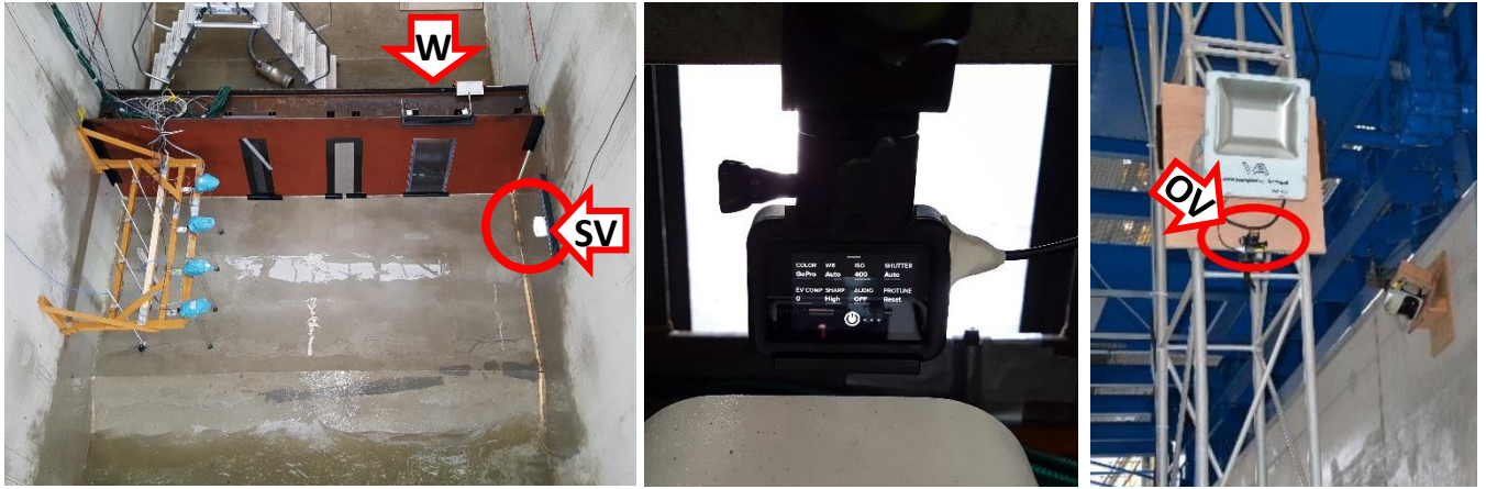
Figure 27: Mounting positions of GoPro cameras. Left: an image from the overview camera (OV) showing the promenade. Cameras marked in red. W denotes window camera (hidden behind the wall), SV – side view camera, and OV – overview camera. Centre: window camera as seen from behind the wall. Right: the overview (OV) camera was mounted on a frame, which was suspended on the so called 'blue carriage' crane. Adapted from (image-right): Streicher (2017, p. 12)
