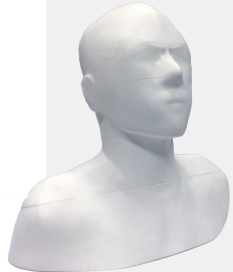
Figure 94 - Adam: 3D printed physical fitting test dummy
