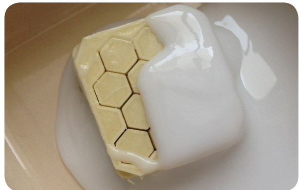
Figure 138 - Fluid silicone mixtures can be in contact with PVA without affecting the material
