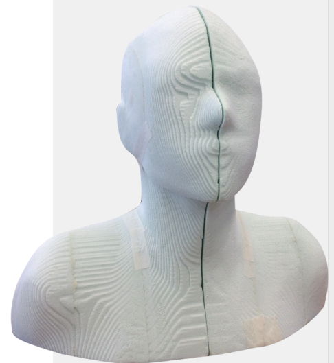
Figure 95 - CNC-milled foam halves of Wally test dummy
