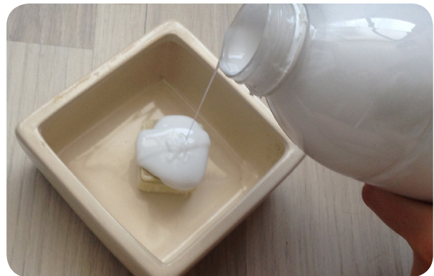
Figure 137 - Pouring silicone mixture into the PVA mould
