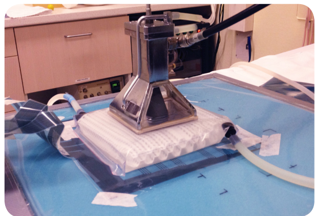
Figure 168 - Set-up of the EM energy conduction experiment
