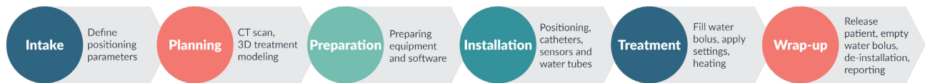
Figure 17 - Phases of the head and neck hyperthermia treatment procedure at the Erasmus MC Cancer Institute
