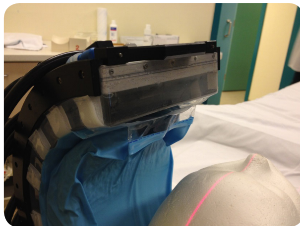
Figure 25 - Air inclusion at the top of the water bolus due to insufficient contact between bolus and applicator
