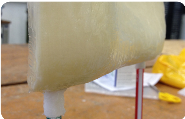
Figure 142 - Brushing thickened silicone mixture onto HoneySkin mould
