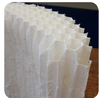
Figure 132 - Printing anatomically shaped HoneyGrids with Flex 45 including support material. Diameters are 15mm, wall thickness 0.4mm and fill 100%
