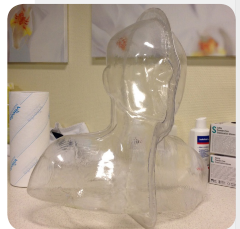
Figure 96 - Wally: Vacuum formed cooling and heating test dummy
