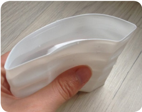
Figure 135 - HoneySkin scale model of 0.35mm thick printed in spiralize mode
