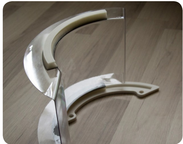
Figure 144 - Prototype of microsuction tape bonding and functionality of the sliding mechanism
