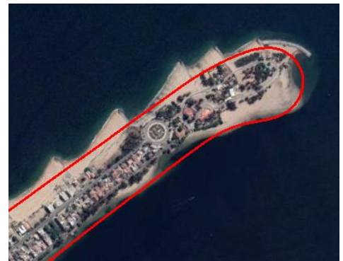
Figure 4-8 – Averaged/ smoothed out coastline used to generate spit bathymetry shown in red
