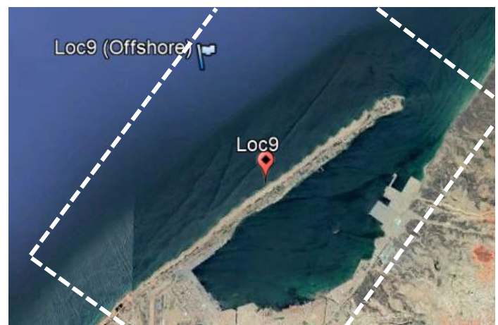
Figure 5-8 – Location of nearshore wave climate (red maker), used for calibrated UNIBEST model and case II and IV in ShorelineS, and offshore wave climate, used for case I and III. Dashed lines indicate boundaries wave model.
