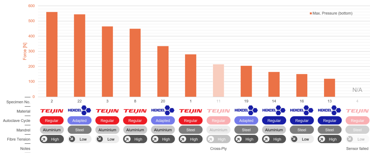
Figure 4.7: Maximum force measured during the autoclave cycles by the respective bottom pressure sensors per specimen in descending order.
