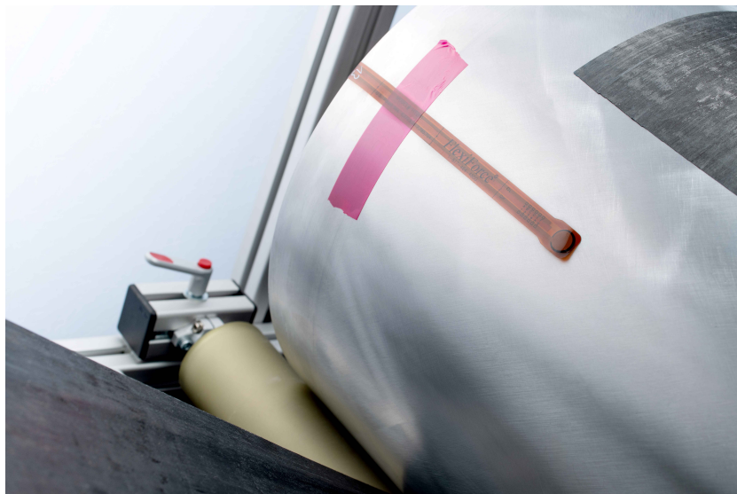
Figure 2.24: Mandrel on manufacturing rig with the first ply about to be wrapped above the pressure sensor.
