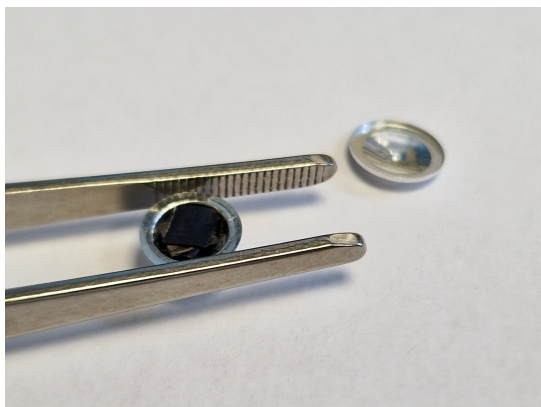
Figure 2.19: Teijin DSC sample in aluminium crucible before closing.
