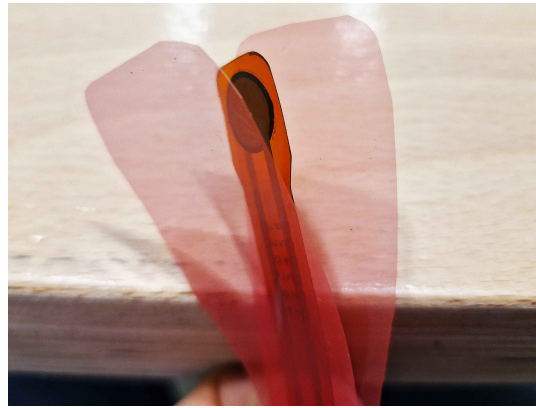
Figure 2.25: Pressure sensor protected by layer of release film (Wrightlon® 5200).
