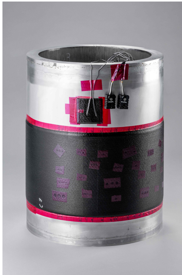
Figure 2.34: Mandrel with quadratic traveller specimen and thermocouples. The large cylindrical specimen on the mandrel was sourced from a different experimental study but was manufactured the same as the specimens for this thesis (DLR).
