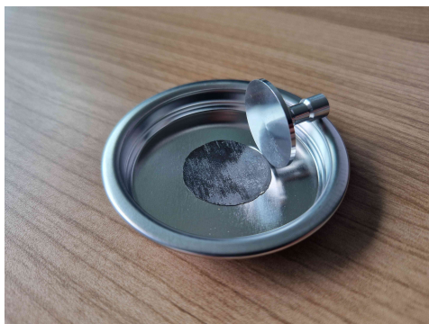
Figure 2.17: Uncured Teijin sample between two parallel plates for rheology study.
