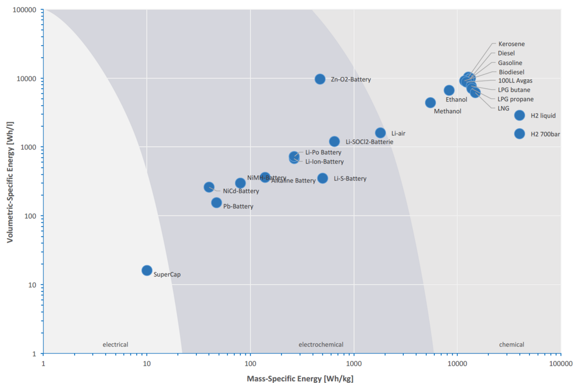
Figure 1.2: Mass- and volumetric-specific energy of multiple energy carriers (Drone Industry Insights, 2017).
