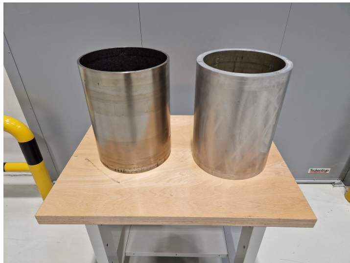
Figure 2.8: Picture of the steel (left) and aluminium (right) mandrel.
