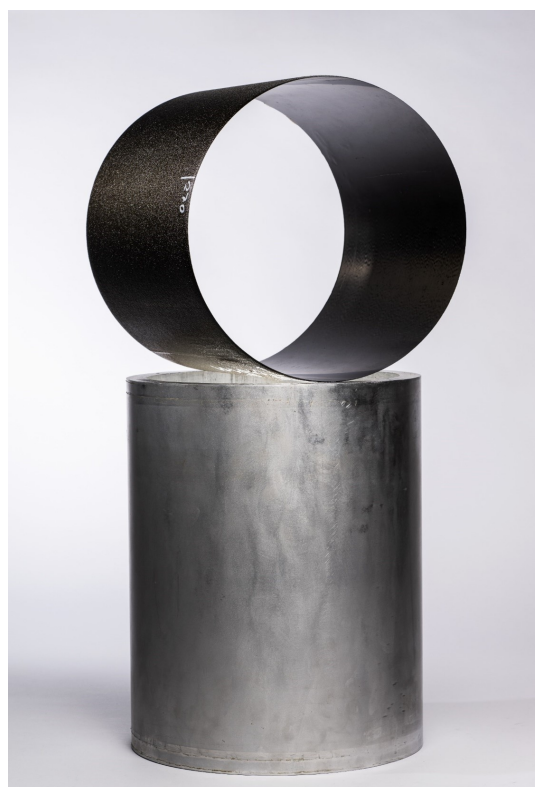
Figure 1.9: Single-curved mandrel made from Aluminium with CFRP probe on top from previous experiments. Diameter 350mm, height 450mm (DLR).
