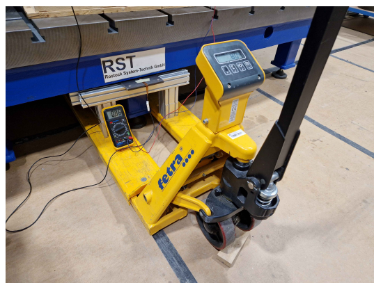
Figure 2.32: Improved sensor calibration with pallet truck for high weight spectrum. The measurement accuracy is sufficient for the use case.
