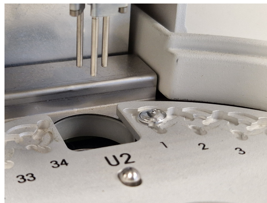
Figure 2.20: Automated sample picking in DSC machine.
