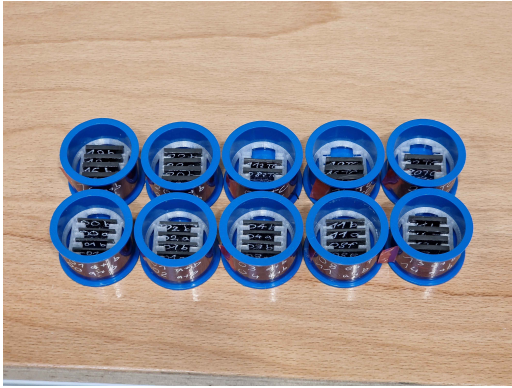
Figure 2.35: Micrograph clamped in custom 3D printed holders inside embedding moulds.
