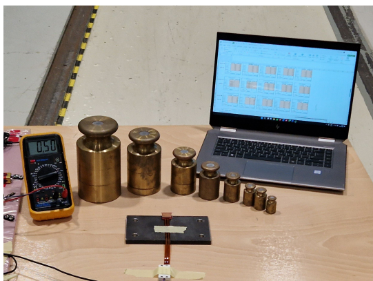
Figure 2.31: Calibration weights for low weight sensor calibration spectrum.
