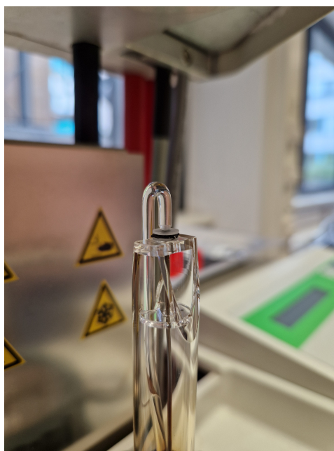
Figure 2.21: Sample between two glass plates in TMA machine for thickness measurement.
