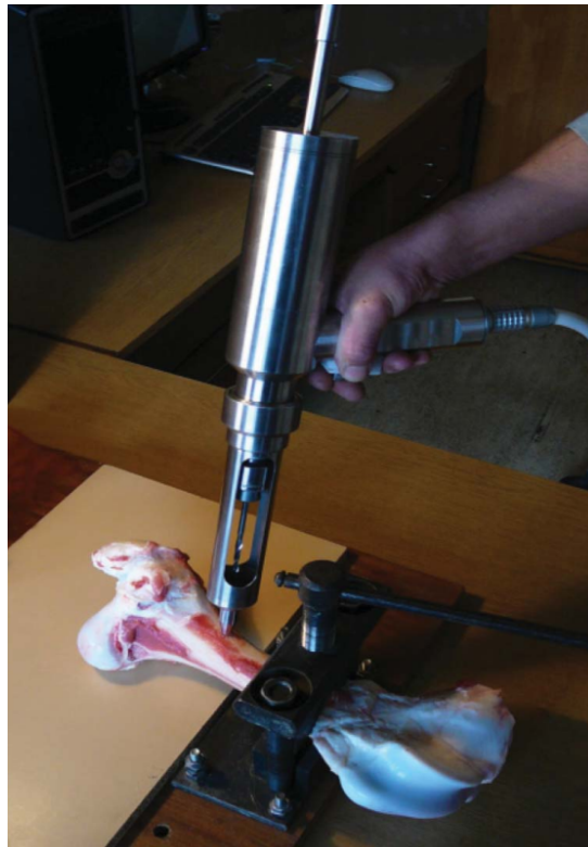
Figure 2: Drilling performed using the ODRO [20] reduces complications, but introduces a very bulky device.
