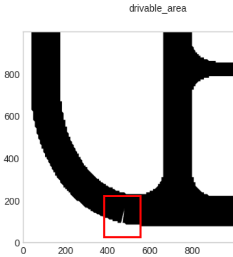
Fig. 10: Imperfections in the map data result in slits/cuts into the lanes which should be eliminated.
