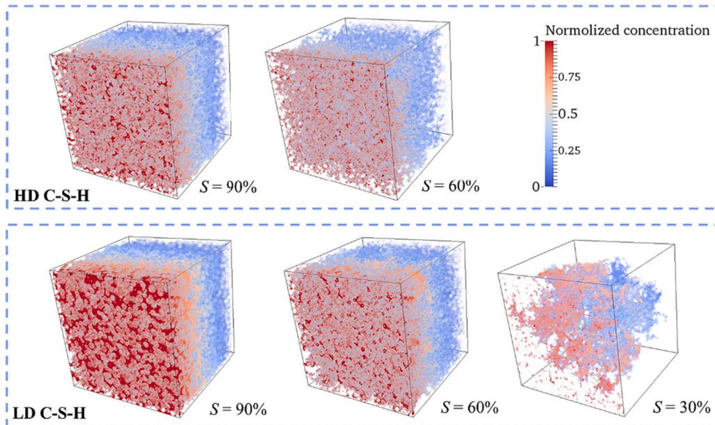
Fig. 19. Steady-state chloride concentration distribution of RVEs at C-S-H level.
