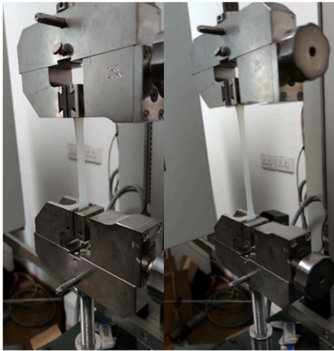
Fig. 11. Tension test under an electronic universal testing machine.
