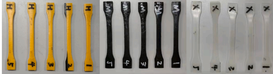
Fig. 10. Dumbbell shape of HDPE (left), MDPE (middle) & XLPE (right).
