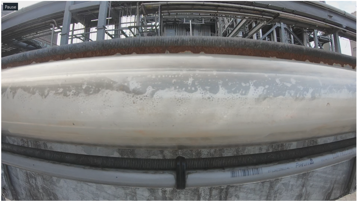
Figure 5.13: Visual observation by the GoPro camera at the end of the flowline for u_{SG} = 5.2 m/s, u_{SL} = 0.3 m/s and 2000 ppm concentration of the surfactant Dreft Original
