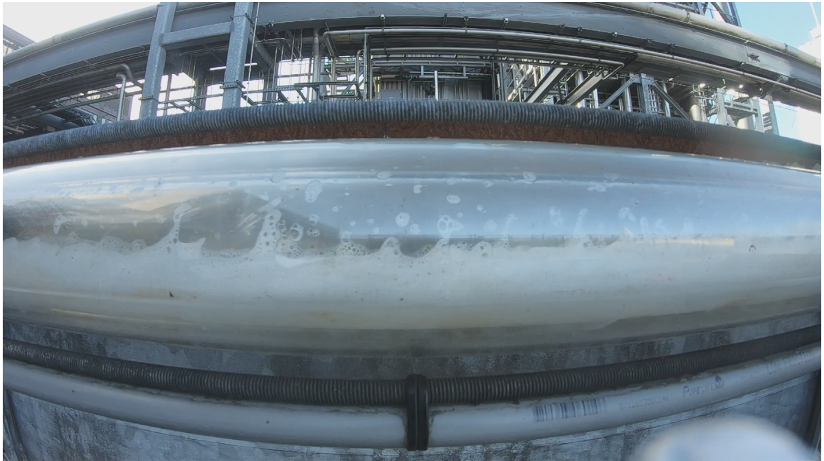
Figure A.3: Visual observation by the GoPro camera at the end of the flowline for u_{SG} = 5.2 m/s, u_{SL} = 0.3 m/s and 1000 ppm concentration of the surfactant Dreft Professional
