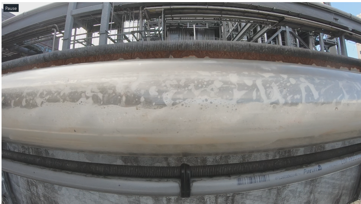
Figure A.4: Visual observation by the GoPro camera at the end of the flowline for u_{SG} = 5.2 m/s, u_{SL} = 0.3 m/s and 1500 ppm concentration of the surfactant Dreft Professional
