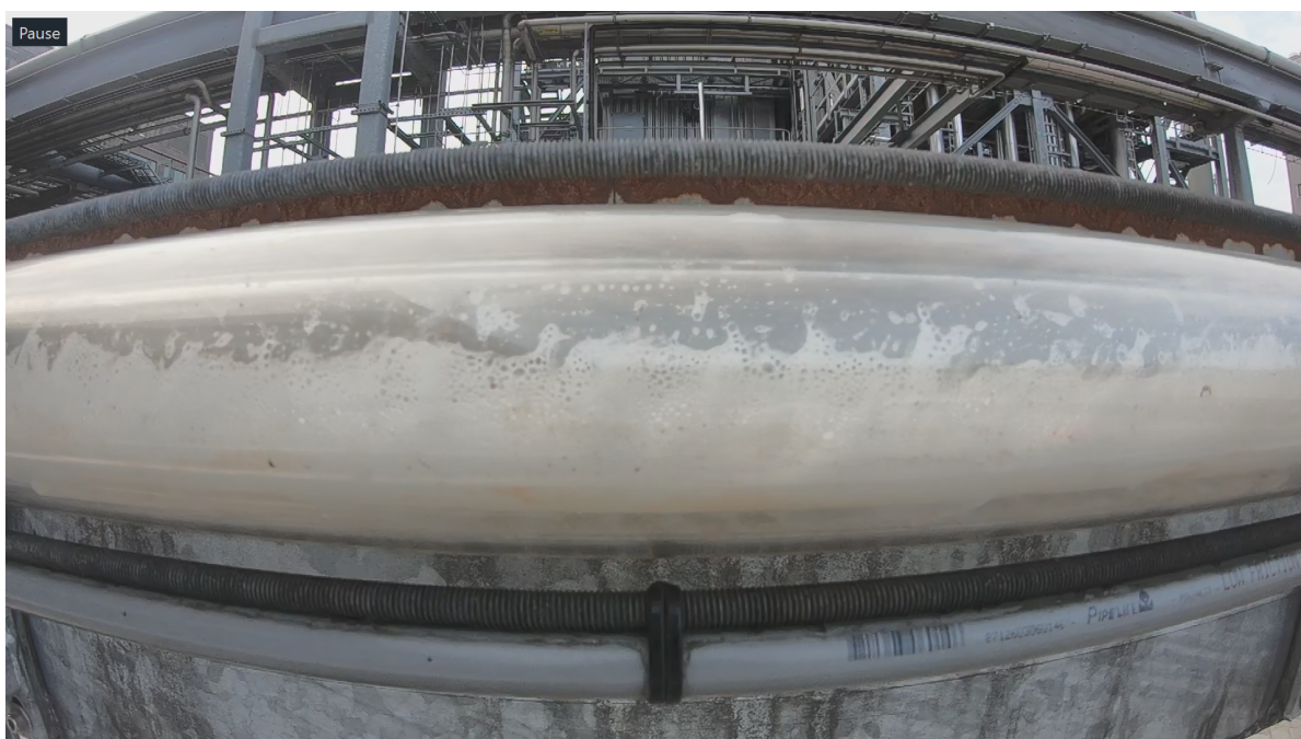
Figure A.5: Visual observation by the GoPro camera at the end of the flowline for u_{SG} = 5.2 m/s, u_{SL} = 0.3 m/s and 2000 ppm concentration of the surfactant Dreft Original
