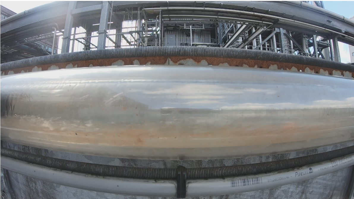
Figure A.1: Visual observation by the GoPro camera at the end of the flowline for u_{SG} = 5.2 m/s, u_{SL} = 0.3 m/s and no surfactant was added
