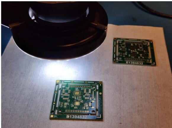
(a) Panelized Bare PCBs being inspected upon delivery
