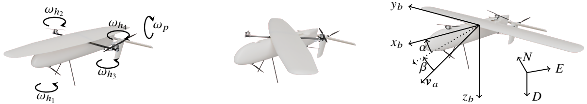
(a) VSQP at \Lambda = 0^\circ , in quad-mode configuration, with the propellers' rotation conventions used.
