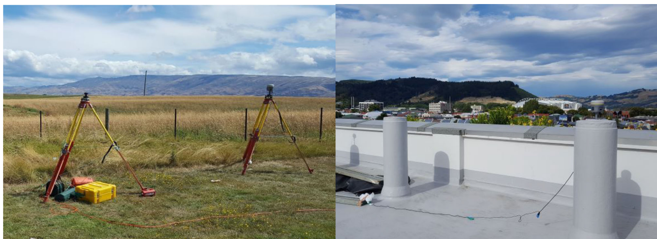
(a) Receiver setup of 112.9 km baseline
