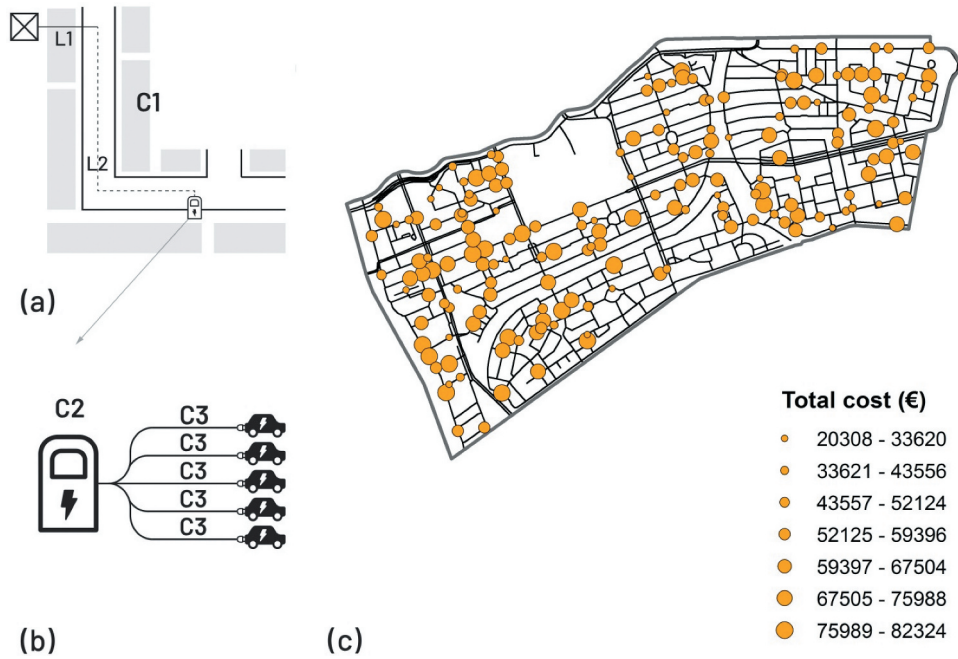
Figure 3. The cost of a new semi-fast charger at a candidate location account for cost of cabling to electricity substation (a) and cost of a semi-fast charger with 5 plug-ins (b). The overall cost is calculated and mapped for each of the 180 candidate locations (c).
