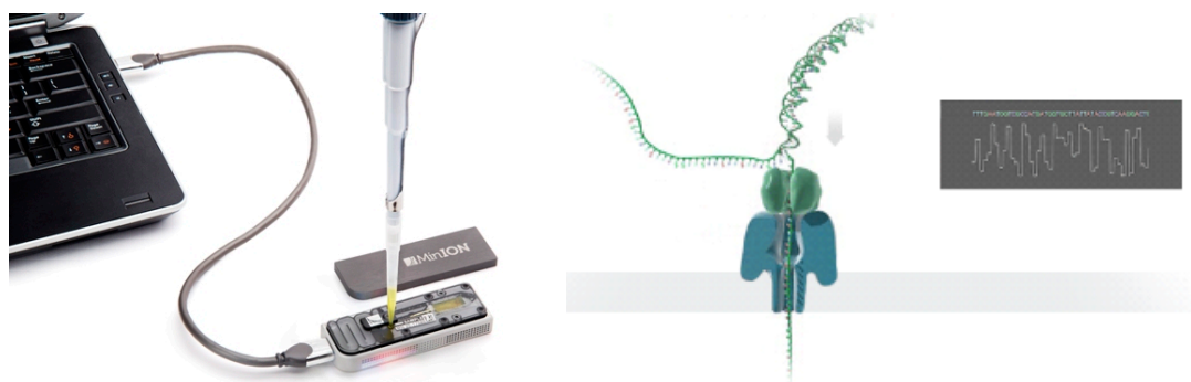
Figure 8.1. MinION sequencing. A protein nanopore is set in an electrically resistant polymer membrane and an ionic current is passed through it. After the DNA sample is added to the flow cell the current is disrupted as the nucleotide bases pass through in different combinations, measured by a sensor. The data streams are passed to an integrated circuit and a software that generates the signal-level data. Adapted from: nanoporetech.com, 2017
