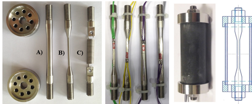
Fig. 2. Three types of restraints; A) thick steel bar, B) thin steel bar and C) spring.
