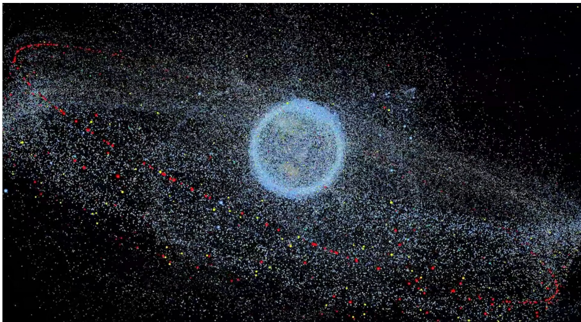
Figure 2.1: Representation of tracked space debris larger than 1mm. Satellites (red), rocket bodies (yellow), fragments (blue) and auxiliary mission-related objects (green) and shown. Courtesy of European Space Agency.
